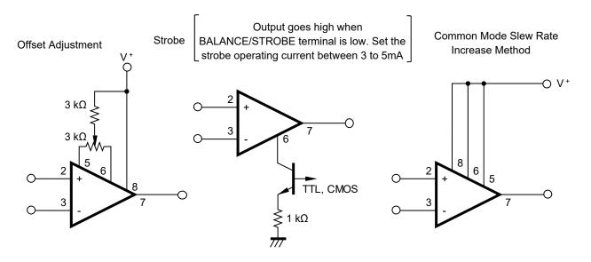
Note Use either pin 5 and pin 6 open (no offset adjustment), the offset adjustment circuit, the strobe circuit (pin 5 open) or the common mode slew rate increase method as shown in above figures. In other cases, malfunction, characteristic deterioration or damage may occur.
