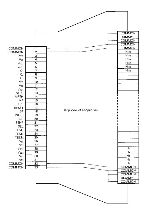
Caution This figure indicates the pin configuration of the standard TCP and does not specify the dimensions of the TCP.
