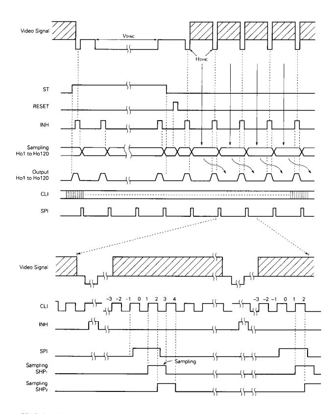
ST: By inputting this signal during the vertical blanking period, the power consumption can be reduced.
