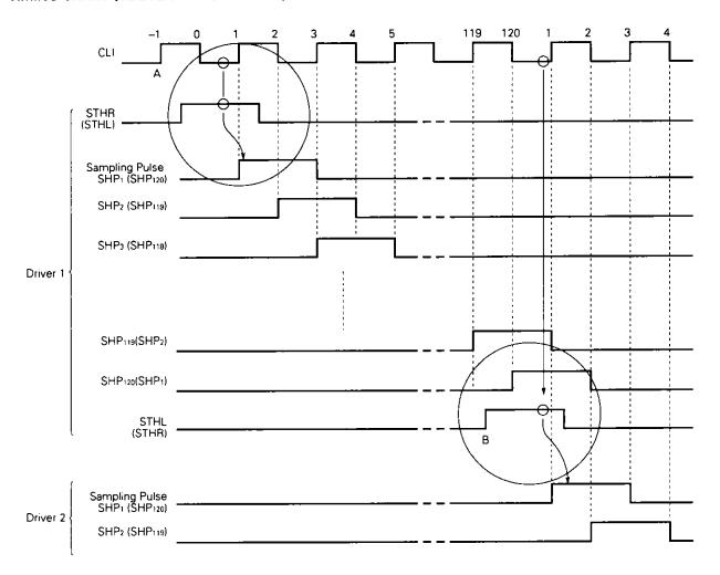
Remark The sampling pulse is set to the first stage of the shift register by the INH input. The shift register is started by the start trigger pulse that is generated when CL1 is low and STHR (STHL) is high, and is stopped when STHL (STHR) is output. STHR (STHL) is input three clocks after INH has fallen.
