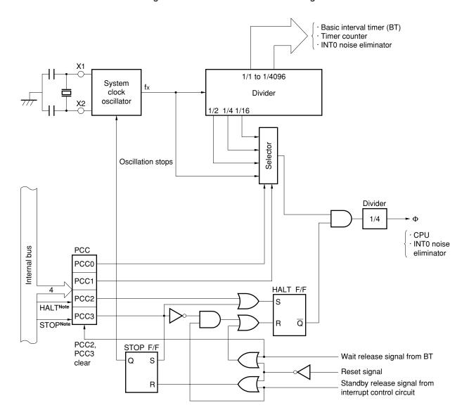
Figure 6-1. Clock Generator Block Diagram
