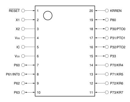
IC: Internally Connected (Connect directly to VDD)
