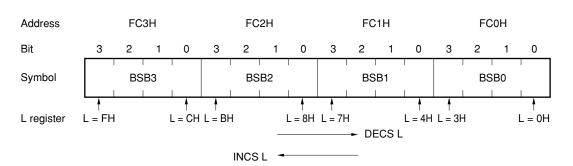
Figure 6-6. Bit Sequential Buffer Format
