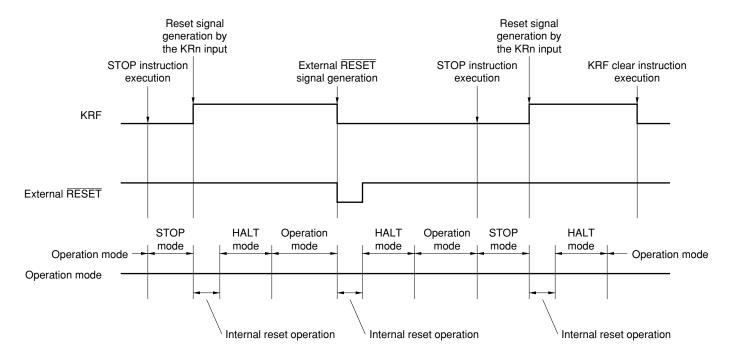
Figure 9-4. KRF Operation in Generating Each Signal
