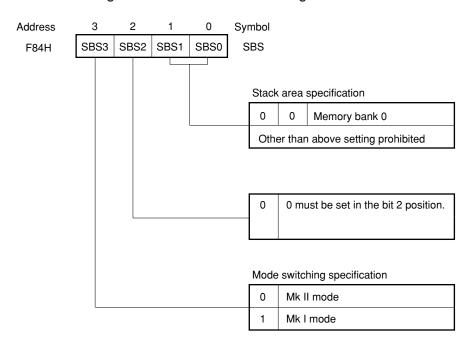
Figure 4-1. Stack Bank Select Register Format
