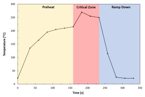
Figure 14. Typical Solder Profile
