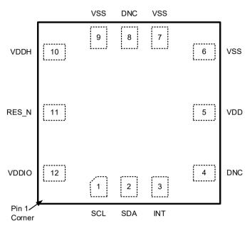
Figure 4. Pin Assignments for 12-LGA Module - Top View
