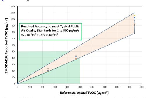
Figure 5. TVOC Measurement According to Typical PBAQ Standards using ZMOD4410
