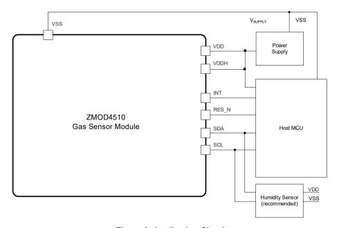
Figure 3. Application Circuit
