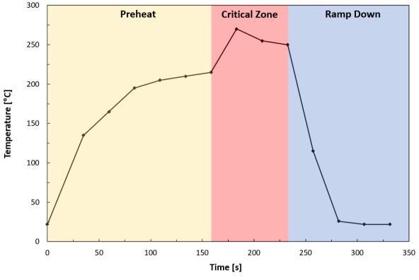
Figure 6. Typical Solder Profile
