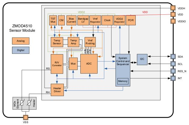
Figure 2. Block Diagram
