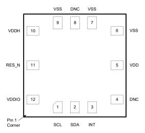
Figure 4. Pin Assignments - Top View
