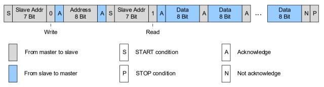
Figure 7. I<sup>2</sup>C Data Transmission Protocol
