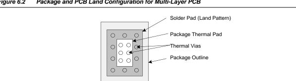
Figure 6.2 Package and PCB Land Configuration for Multi-Layer PCB
