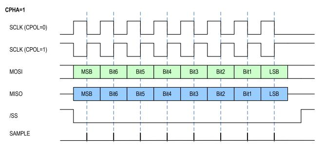
In SPI Mode, each command except NOP is started as shown in Figure 3.7. After the execution of a command (busy = 0), the expected data can be read as illustrated in Figure 3.8 or if no data are returned by the command, the next command can be sent. The status can be read at any time with the NOP command (see Figure 3.9).
