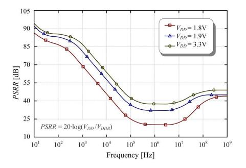
1.4 Power Supply Rejection Ratio (RSRR) versus Frequency
