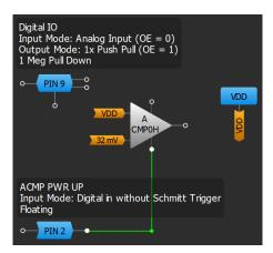
Figure 2: GreenPAK Input Structure Test Schematic
