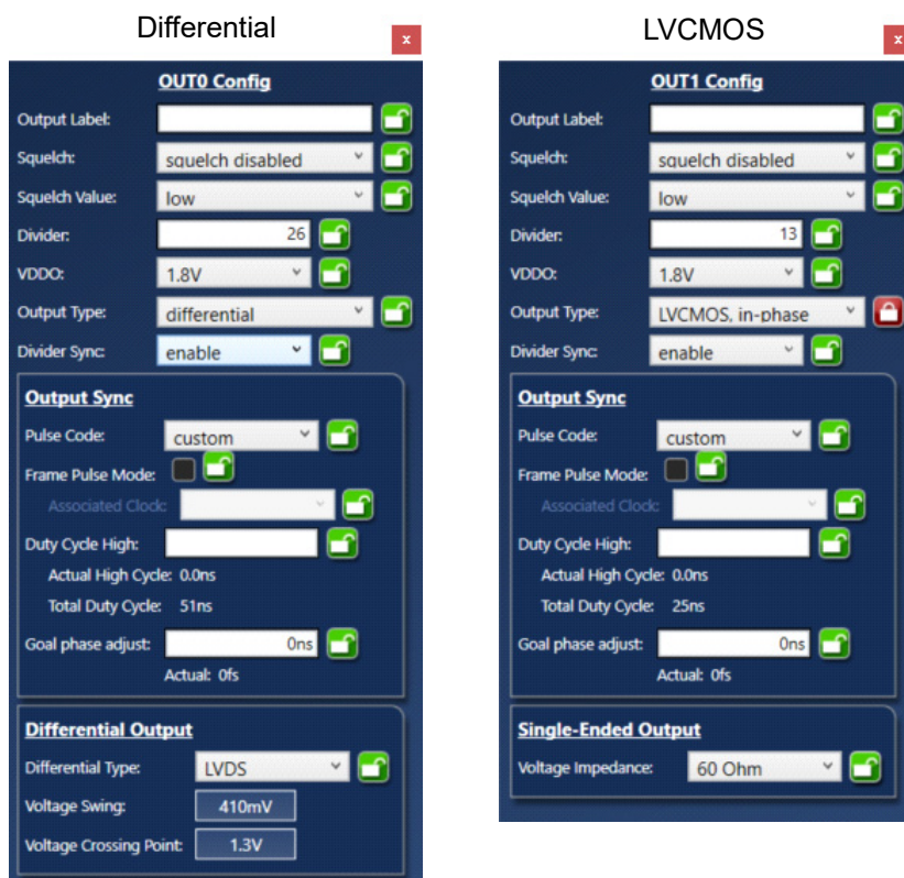
Figure 15. Output Stages – Differential and LVCMOS Signals Windows
