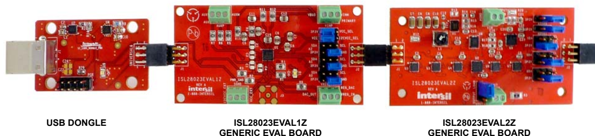
FIGURE 1. ISL28023 EVALUATION KIT EVALUATION BOARDS
