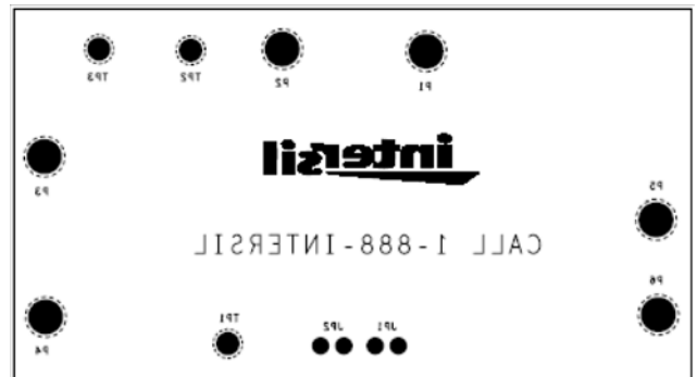
FIGURE 20. ISL6445EVAL3Z - BOTTOM LAYER (SILKSCREEN)
