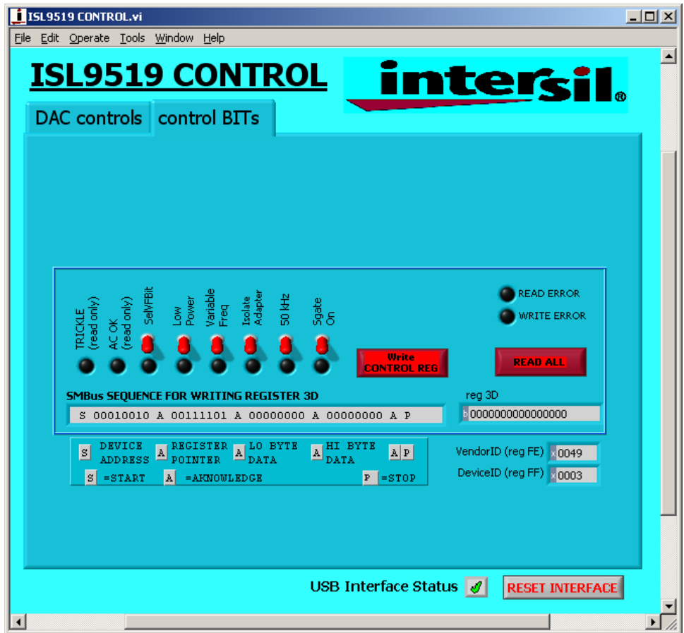
FIGURE 14. CONTROL BITS TAB FOR WRITING THE CONTROL REGISTER
