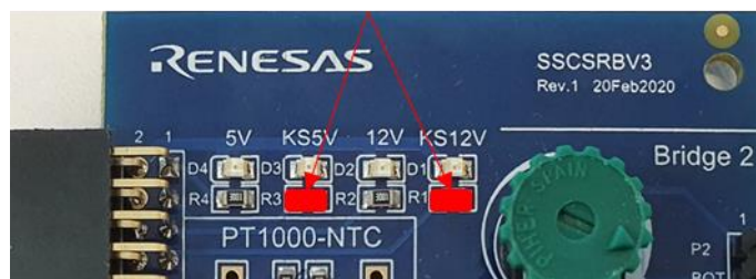
Figure 130. 2-Wire Current Loop SRB3 Specific Configuration
