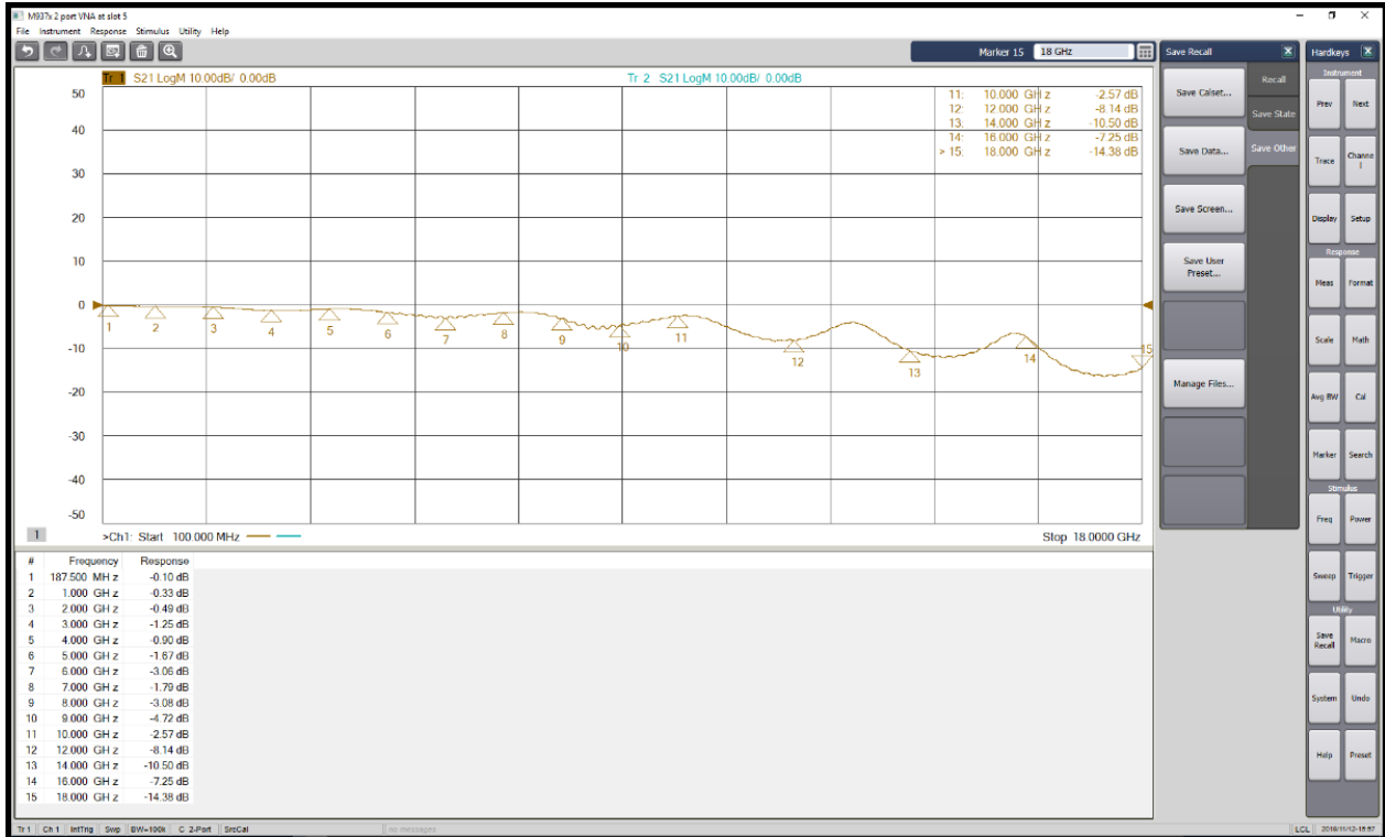
Figure 14. 8V97003 EVB Revision C Transmission Line Loss
