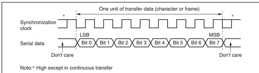
**Figure 13.14 Data Format in Synchronous Communication (For LSB-First)**
