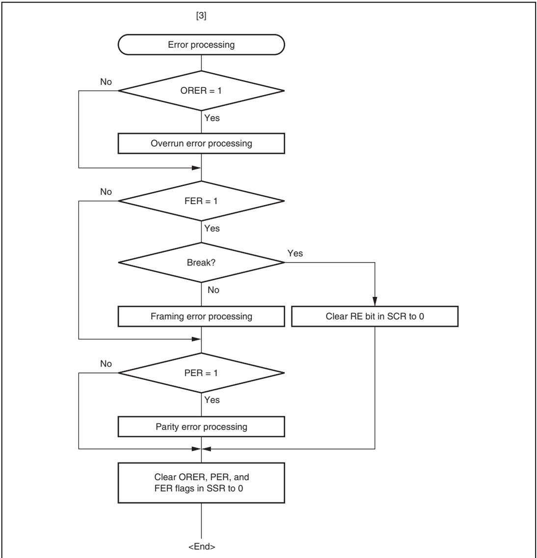
**Figure 13.9 Sample Serial Reception Data Flowchart (2)**
