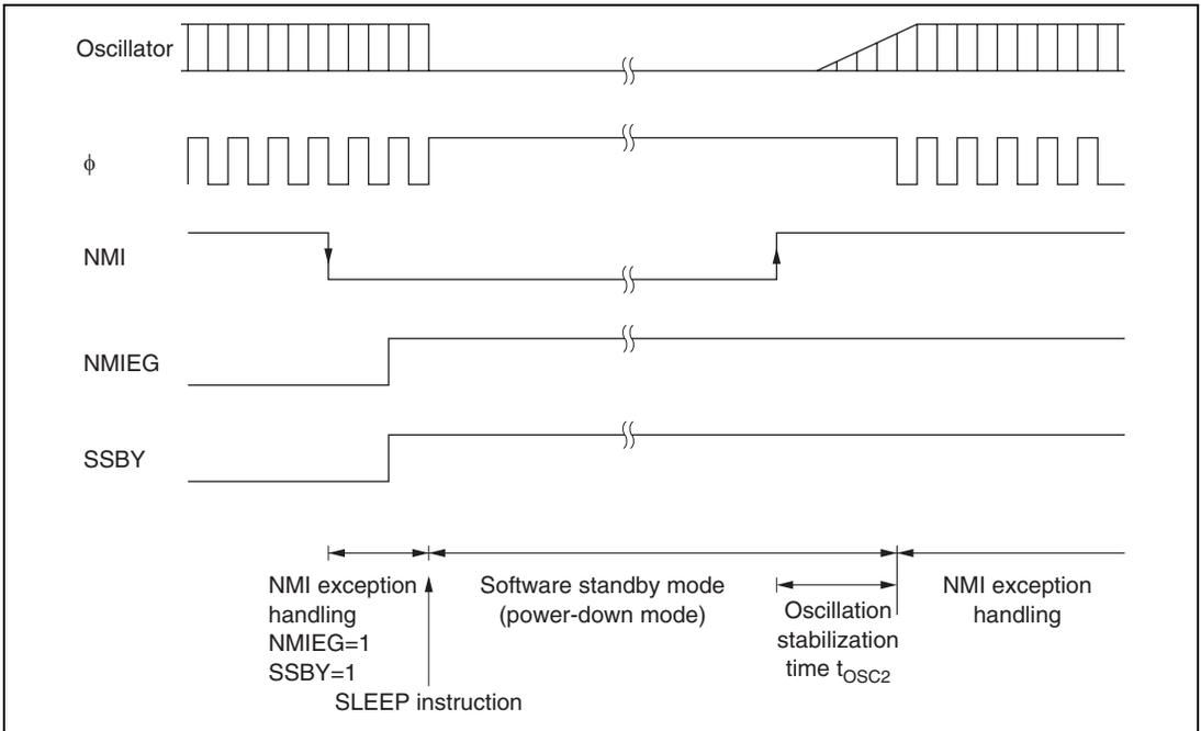
**Figure 21.3 Software Standby Mode Application Example**
