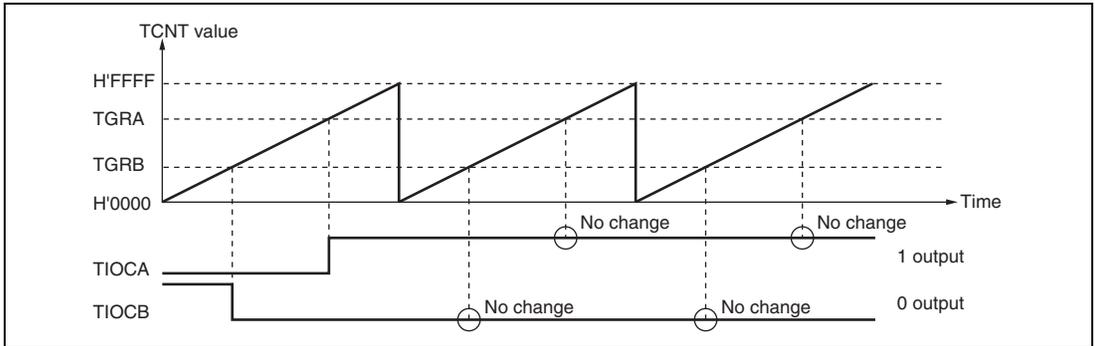
**Figure 10.6 Example of 0 Output/1 Output Operation**
