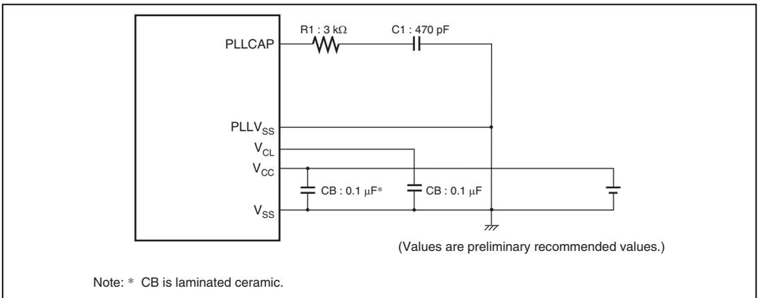
**Figure 20.10 External Circuitry Recommended for PLL Circuit**
