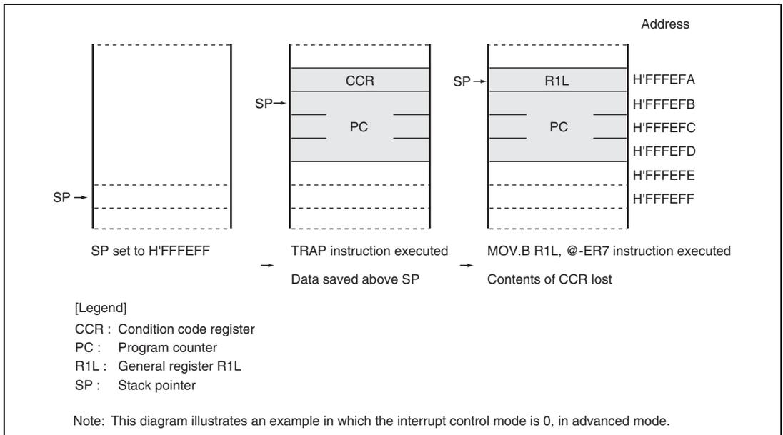
**Figure 4.4 Operation when SP Value Is Odd**
