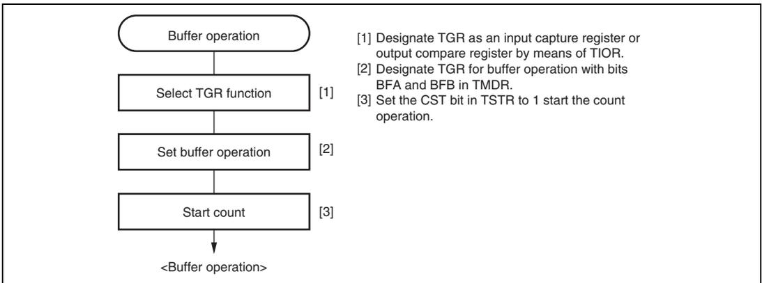
**Figure 10.14 Example of Buffer Operation Setting Procedure**
