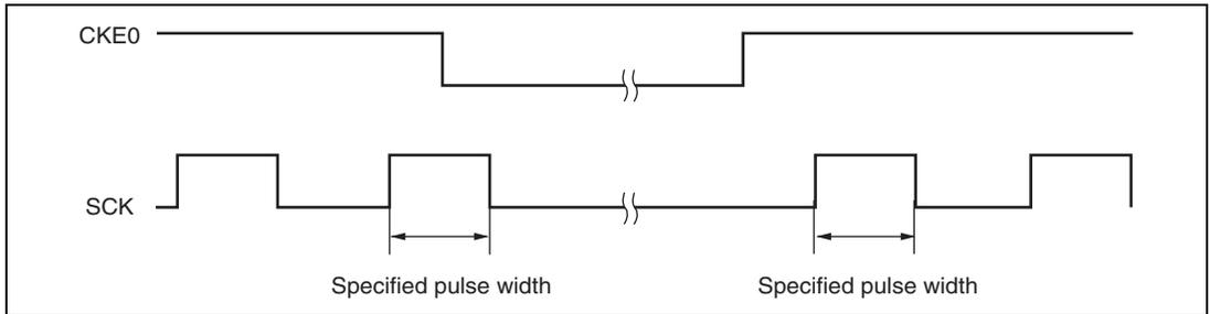
**Figure 13.31 Timing for Fixing Clock Output Level**
