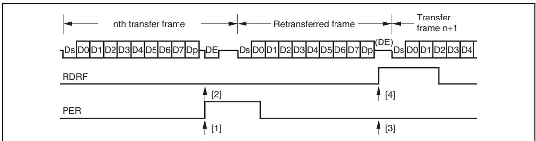
**Figure 13.29 Retransfer Operation in SCI Receive Mode**
