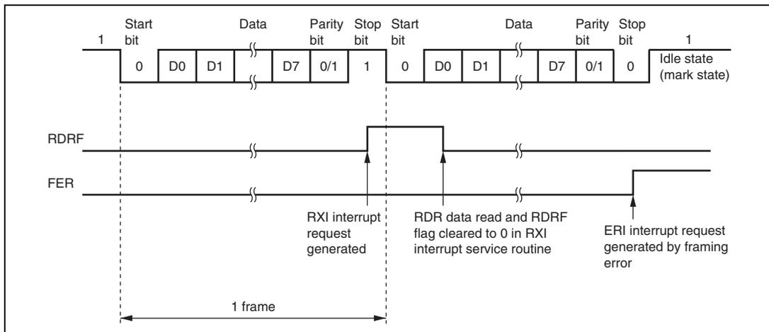
**Figure 13.8 Example of SCI Operation in Reception
