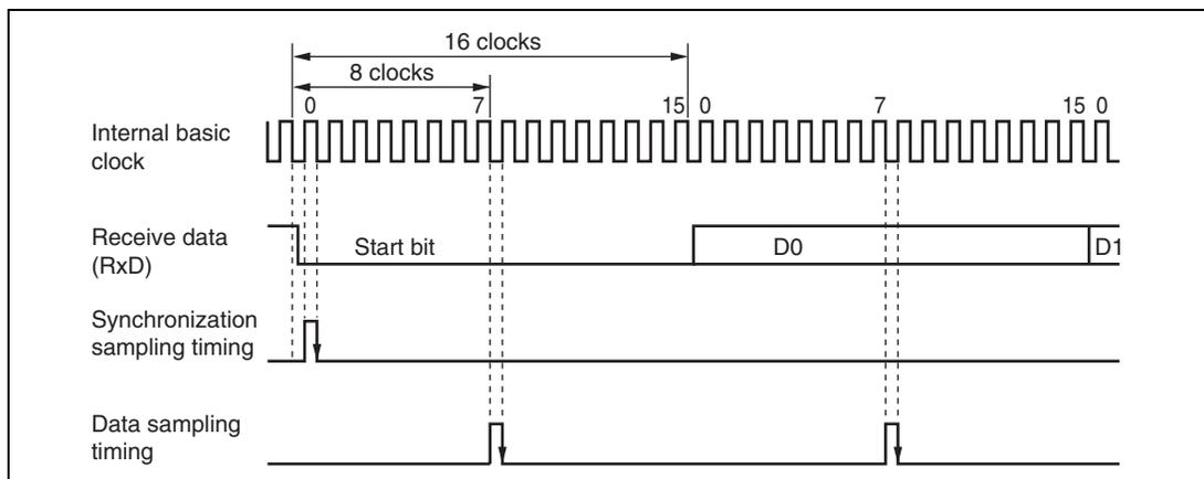
**Figure 13.3 Receive Data Sampling Timing in Asynchronous Mode**
