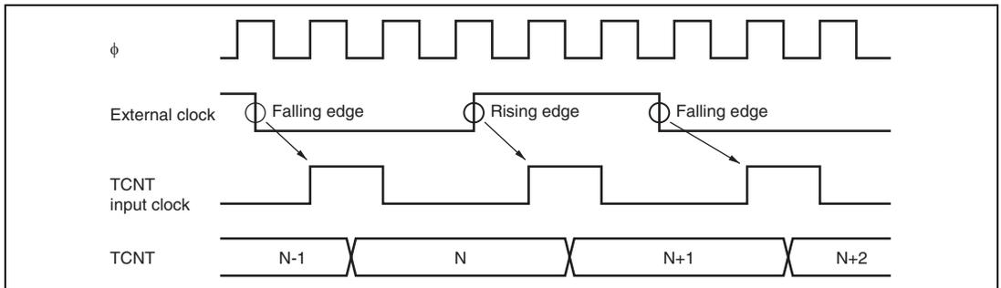
**Figure 10.31 Count Timing in External Clock Operation**
