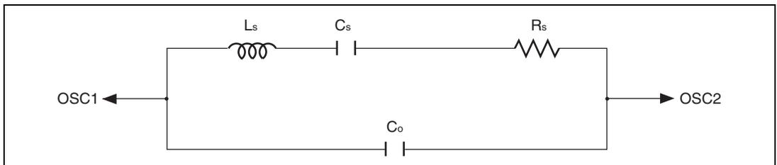
**Figure 20.7 Equivalent Circuit for 32.768-kHz Crystal Resonator**
