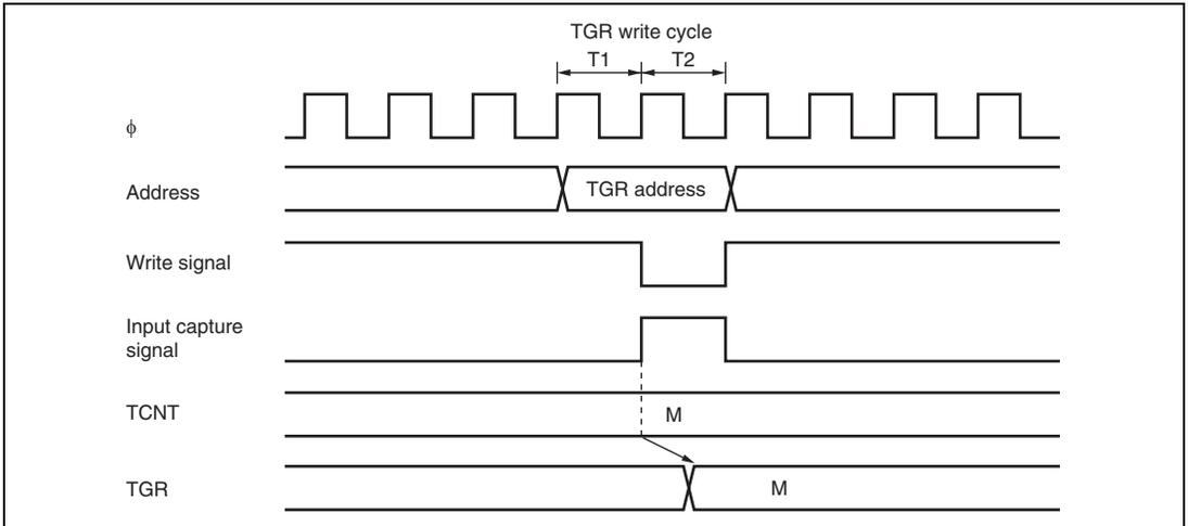
**Figure 10.50 Conflict between TGR Write and Input Capture**
