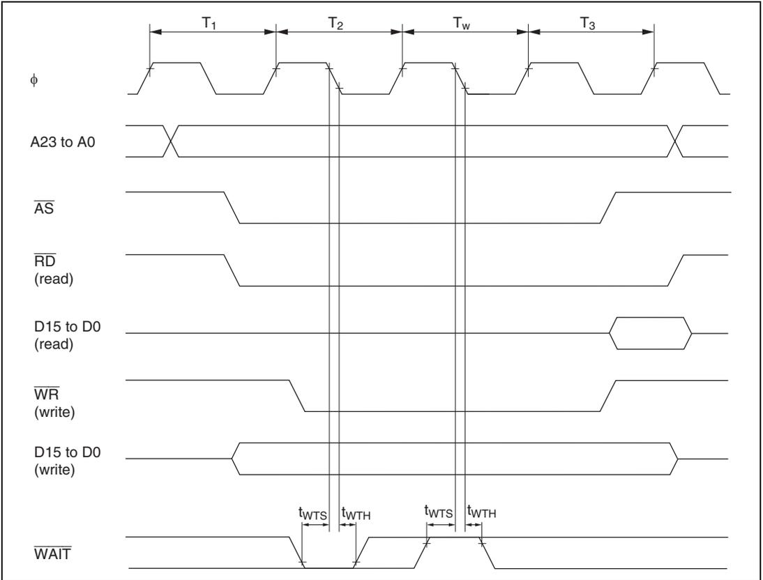
**Figure 23.8 Basic Bus Timing (Three-State Access with One Wait State)**
