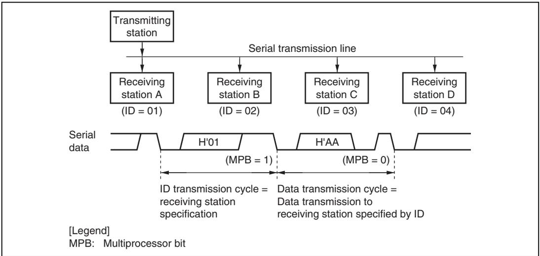
**Figure 13.10 Example of Communication Using Multiprocessor Format
