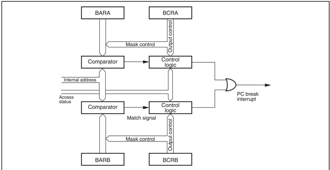
**Figure 6.1** Block Diagram of PC Break Controller
