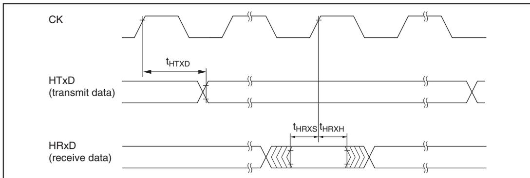
**Figure 23.19 HCAN Input/Output Timing**
