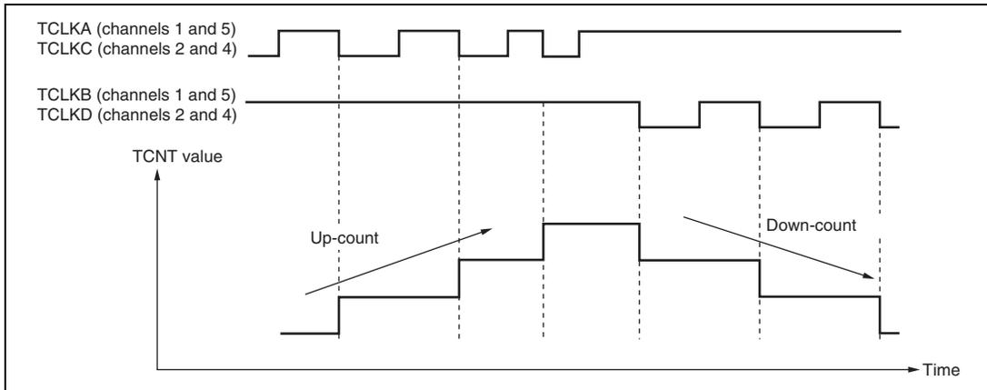
**Figure 10.27 Example of Phase Counting Mode 3 Operation**
