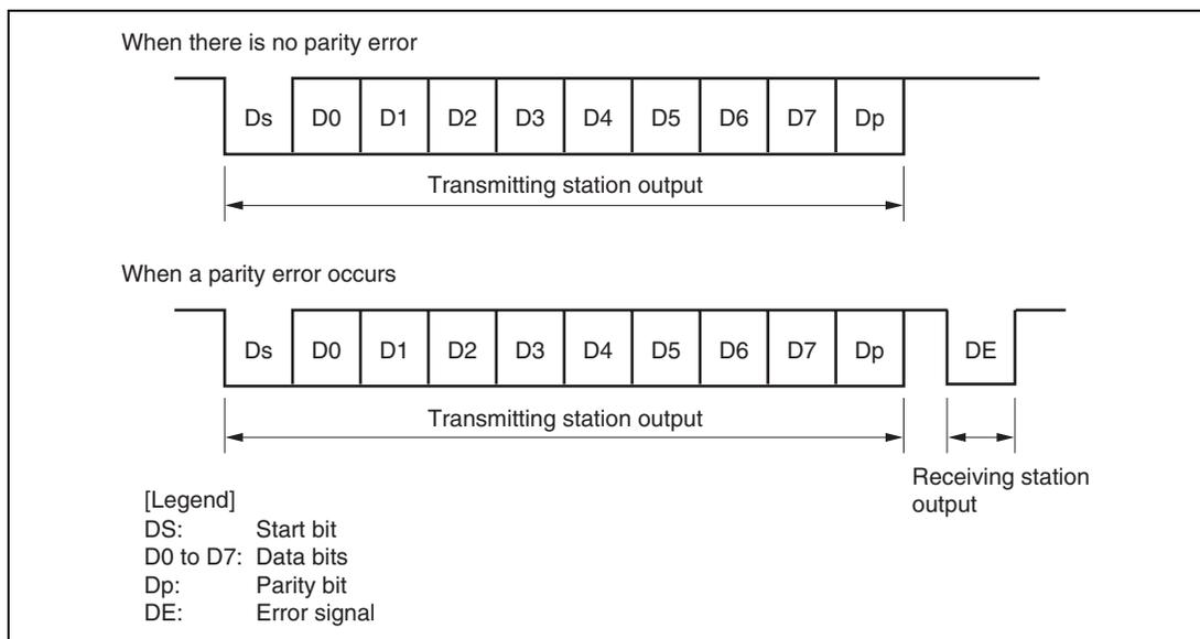
**Figure 13.22 Normal Smart Card Interface Data Format**
