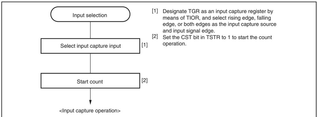
**Figure 10.8 Example of Input Capture Operation Setting Procedure**
