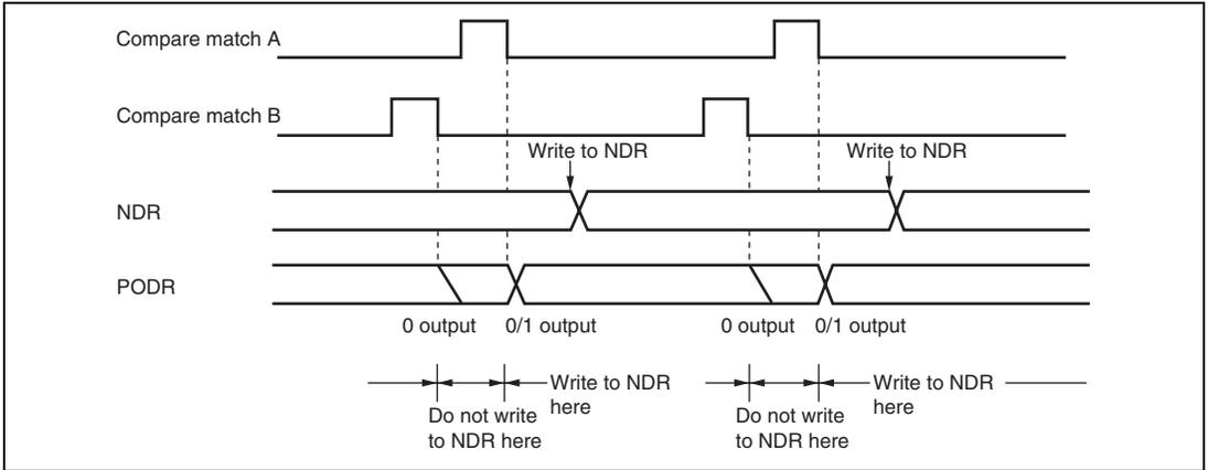
**Figure 11.7 Non-Overlapping Operation and NDR Write Timing**
