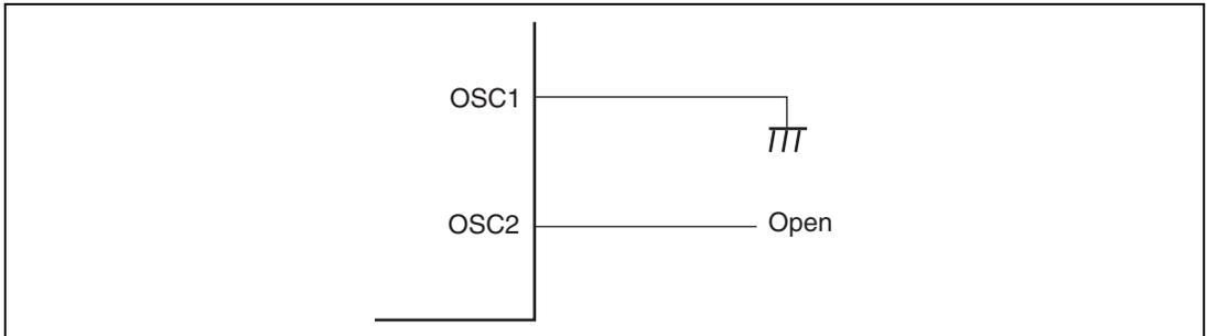
**Figure 20.8 Pin Handling when Subclock is not Used**
