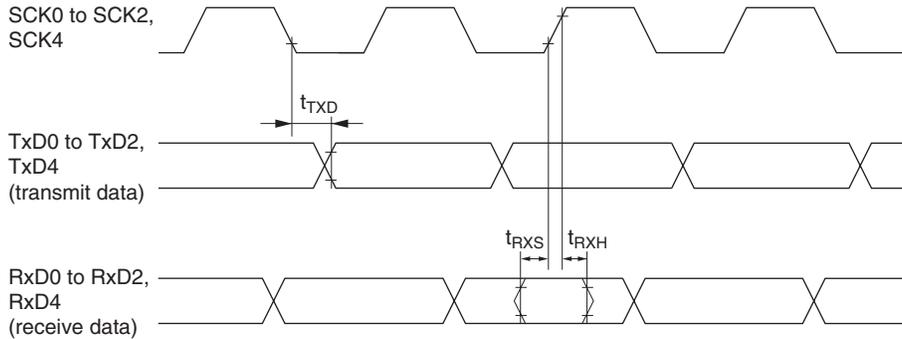
**Figure 23.17 SCI Input/Output Timing (Clock Synchronous Mode)**
