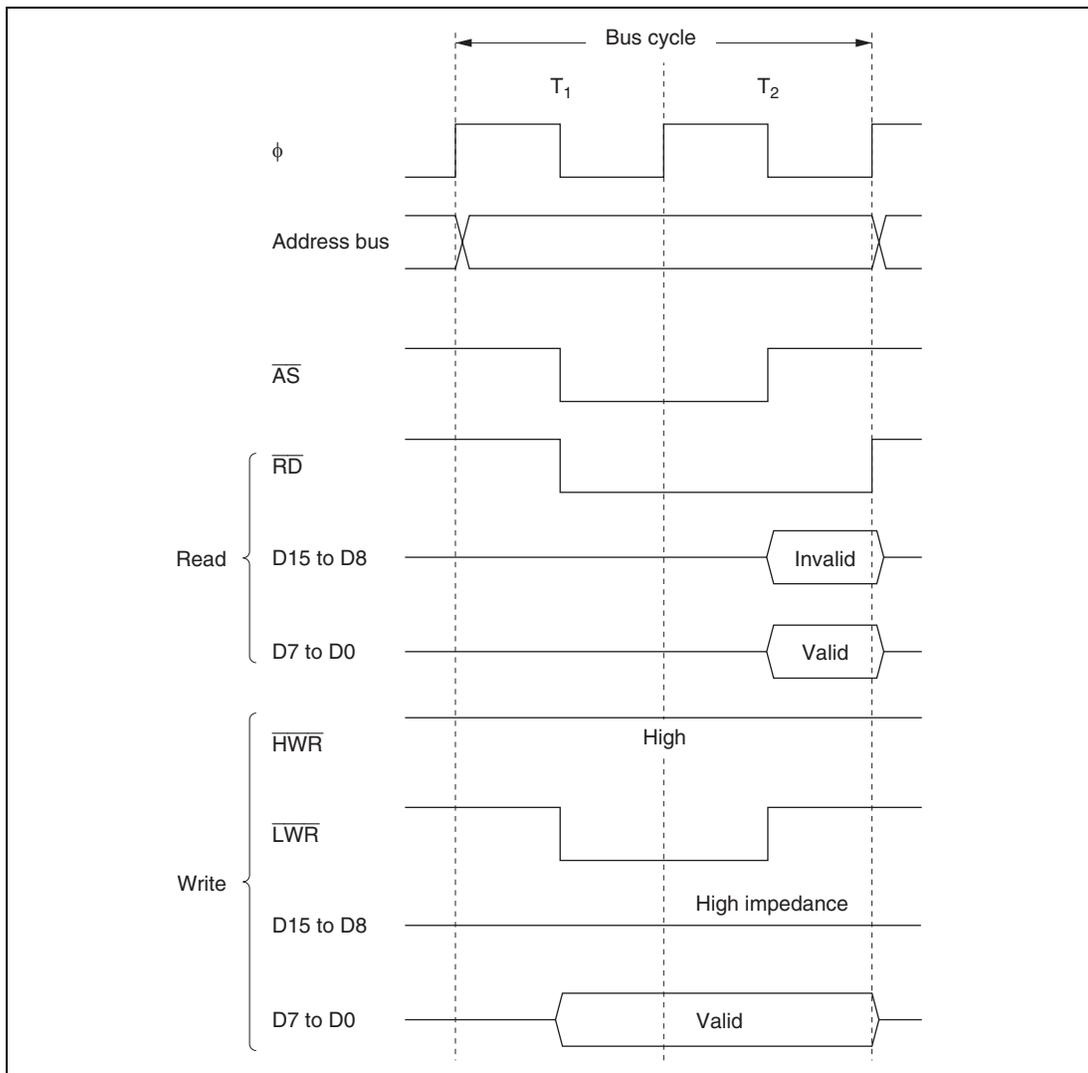
**Figure 7.8 Bus Timing for 16-Bit, 2-State Access Space
