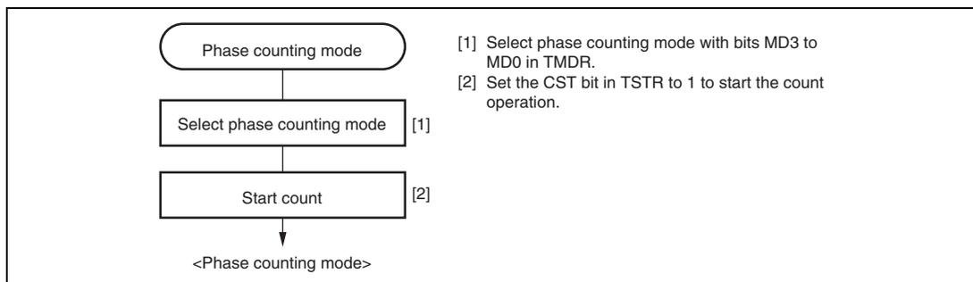
**Figure 10.24 Example of Phase Counting Mode Setting Procedure**
