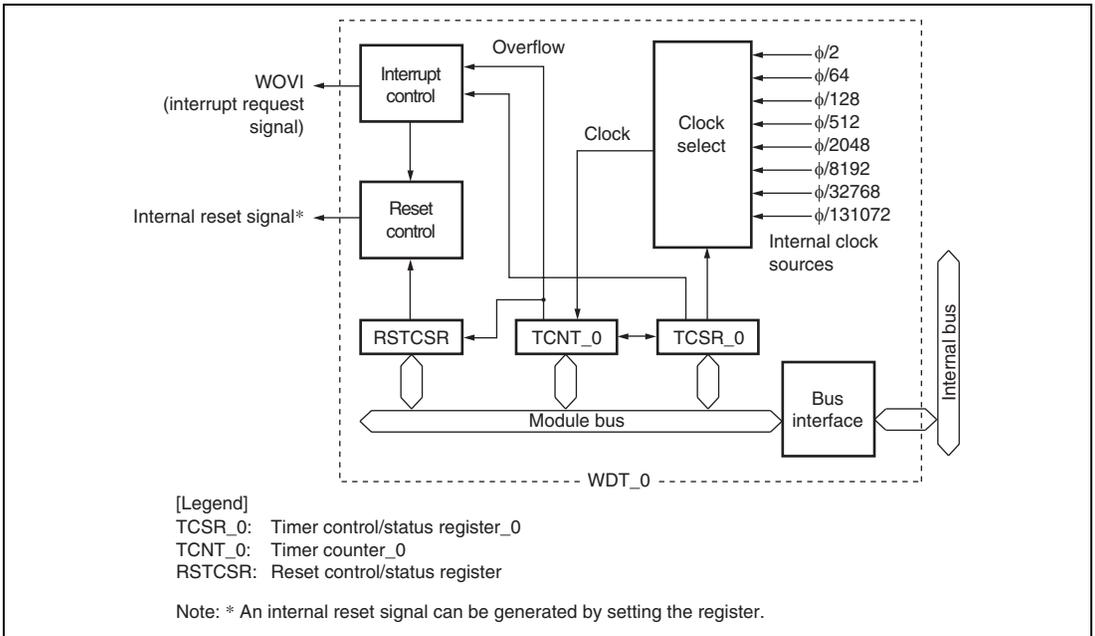
Figure 12.1 Block Diagram of WDT\_0
