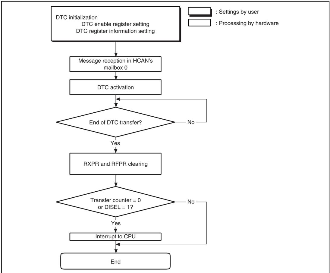
Figure 14.15 DTC Transfer Flowchart
