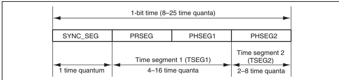
**Figure 14.8 Detailed Description of One-Bit Time**
