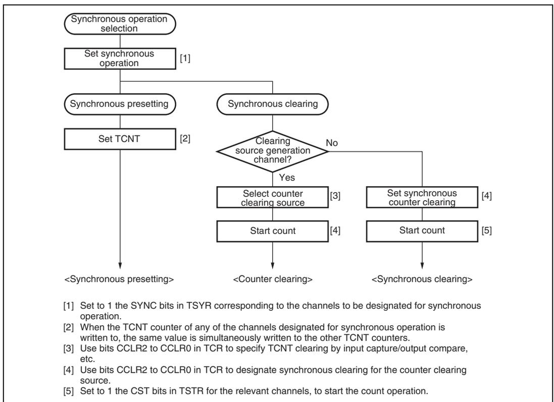
**Figure 10.10 Example of Synchronous Operation Setting Procedure**
