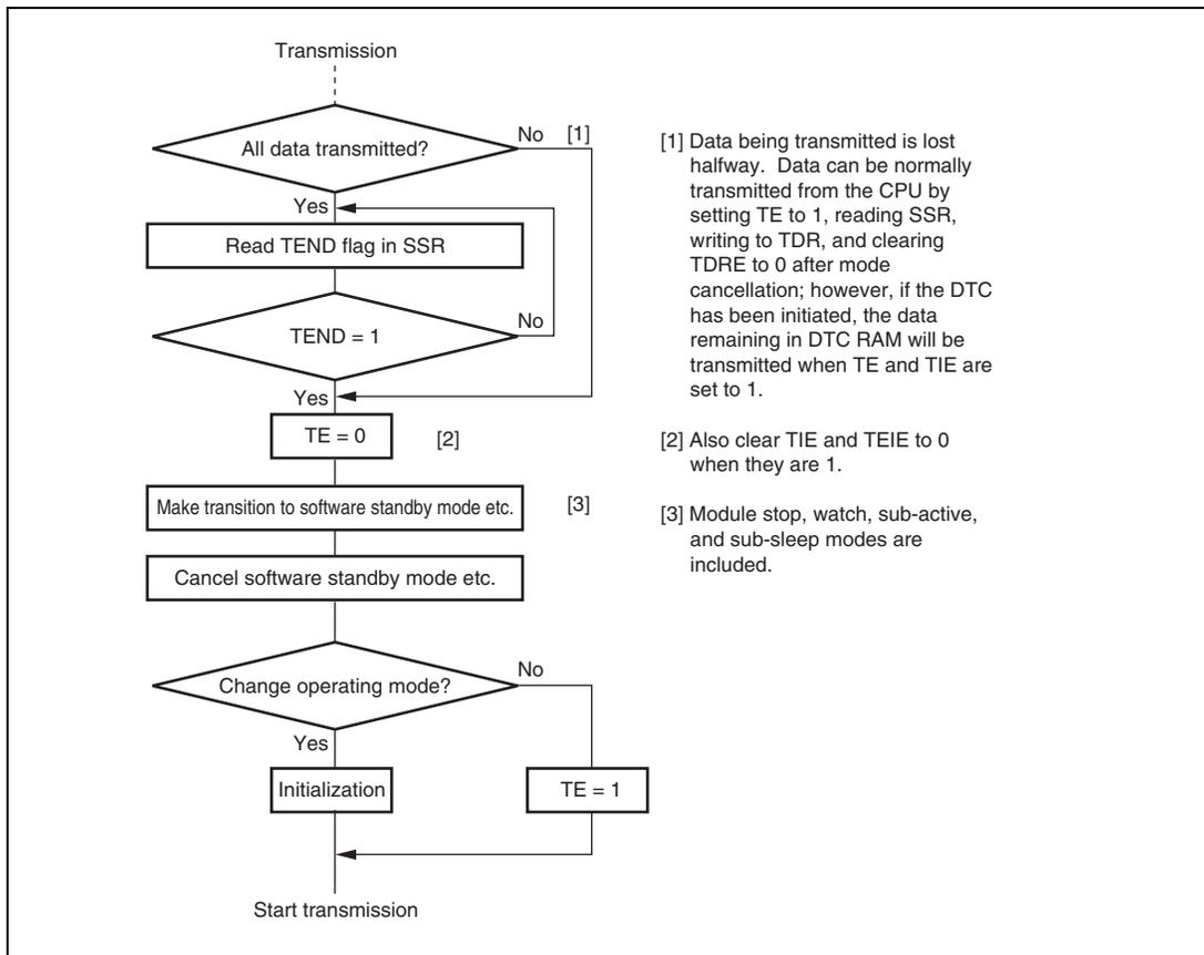
**Figure 13.34 Sample Flowchart for Mode Transition during Transmission**
