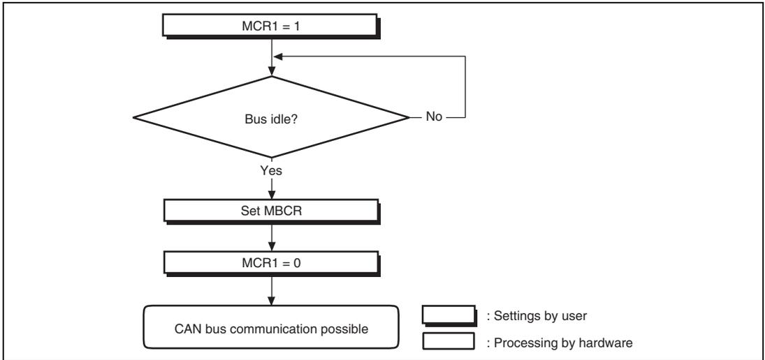
**Figure 14.14 HCAN Halt Mode Flowchart**
