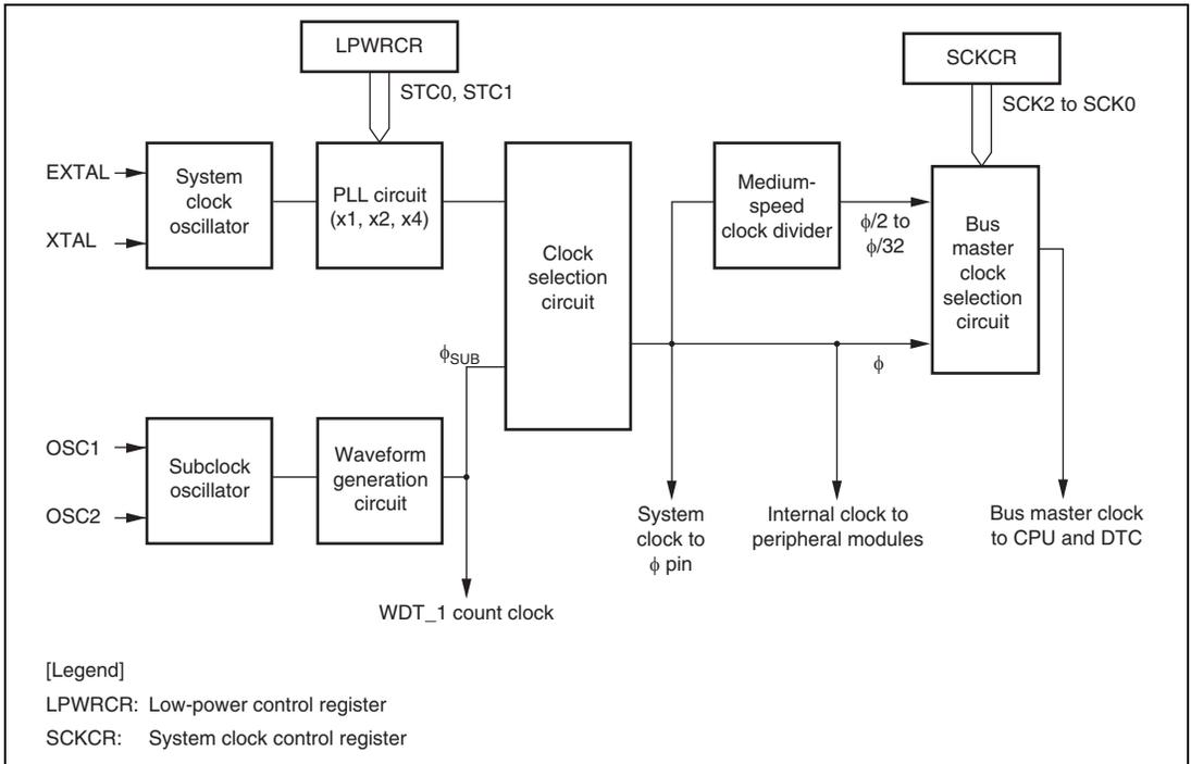
**Figure 20.1 Block Diagram of Clock Pulse Generator**
