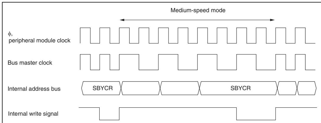
**Figure 21.2 Medium-Speed Mode Transition and Clearance Timing**
