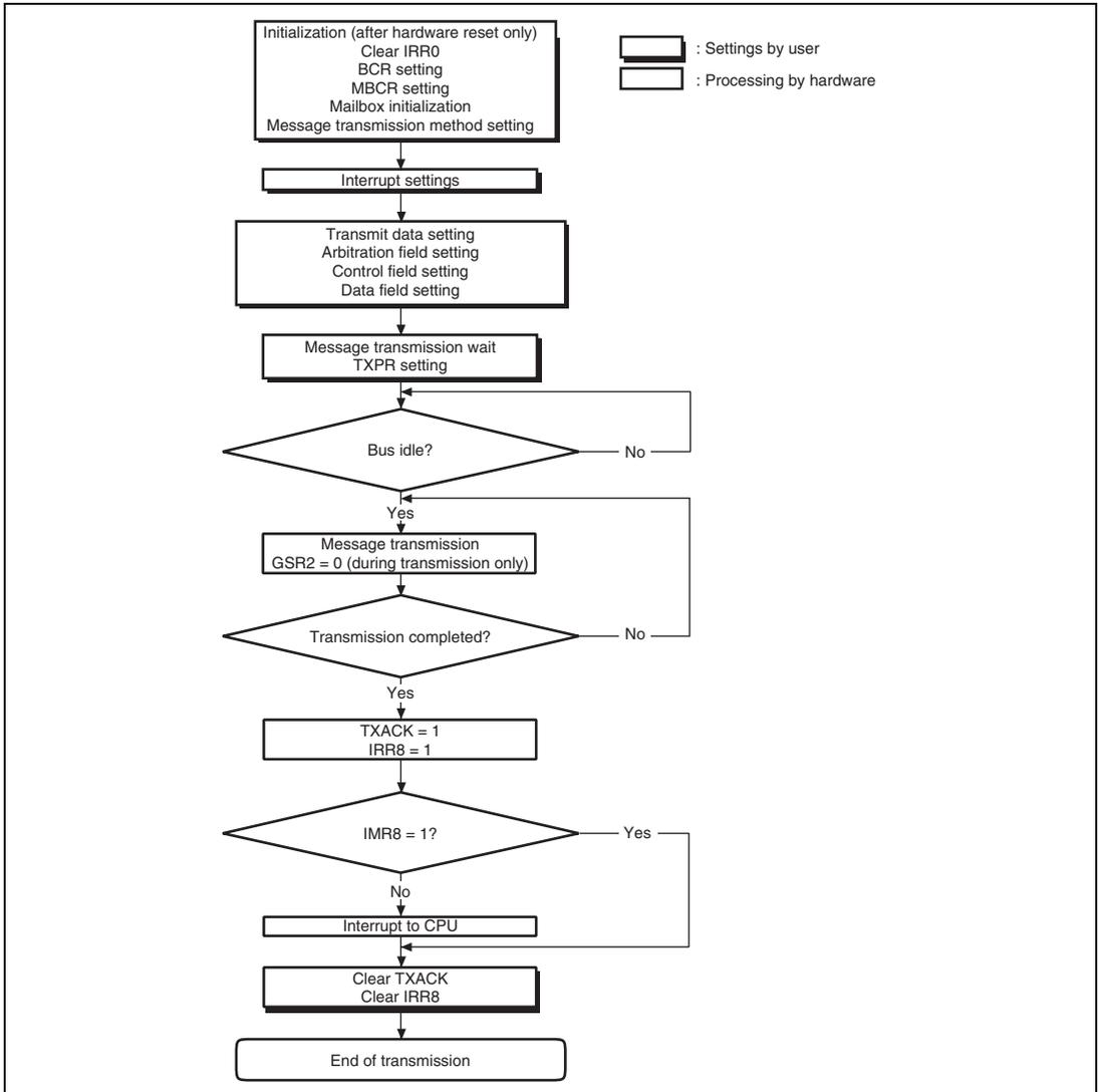
Figure 14.9 Transmission Flowchart
