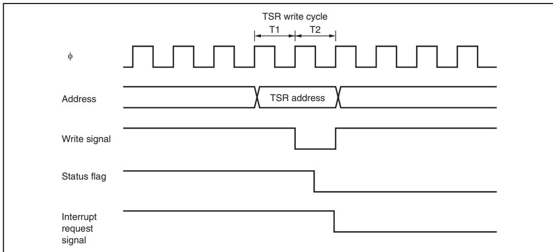
**Figure 10.42 Timing for Status Flag Clearing by CPU**
