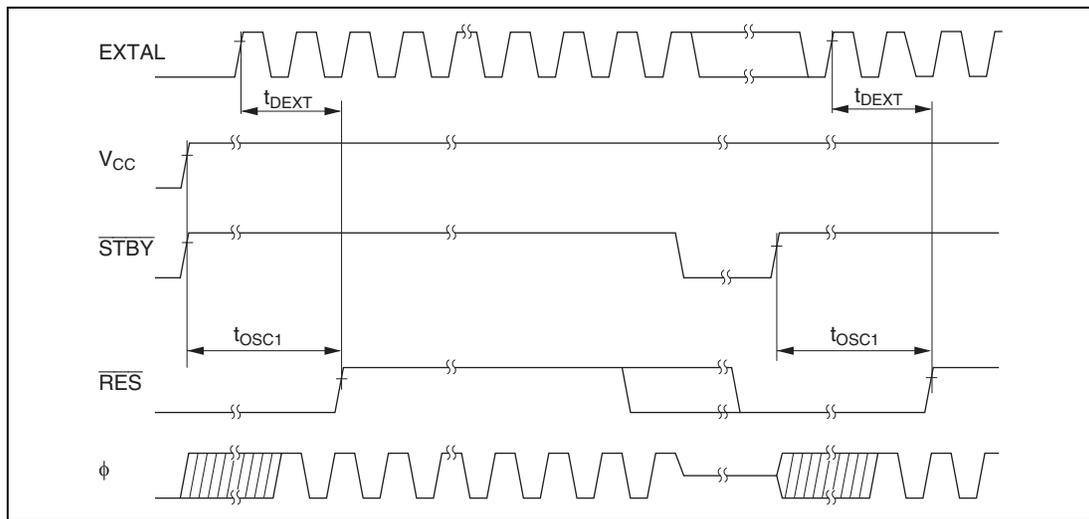
Figure 23.3 Oscillator Settling Timing
