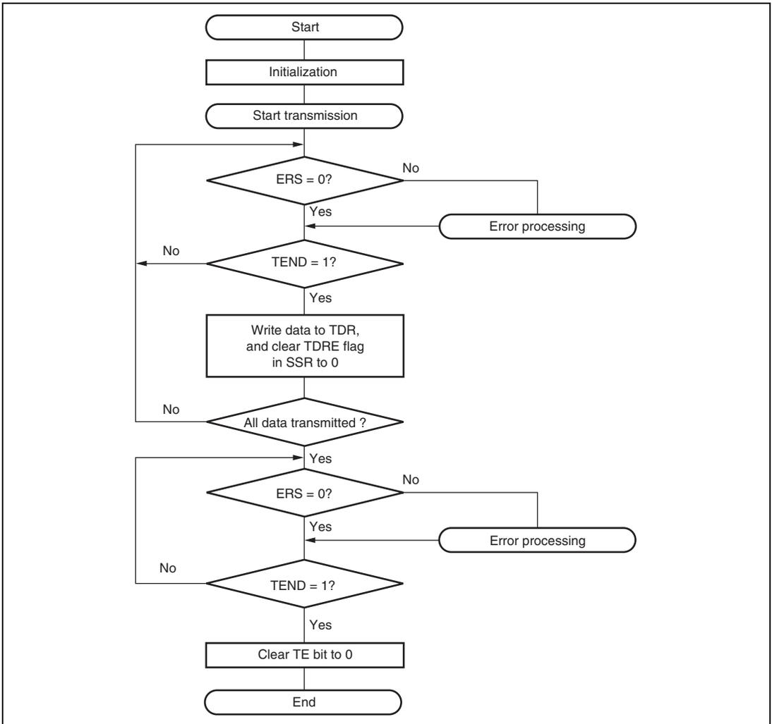
**Figure 13.28 Example of Transmission Processing Flow**
