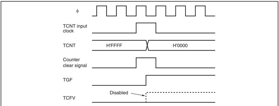
**Figure 10.52 Conflict between Overflow and Counter Clearing**
