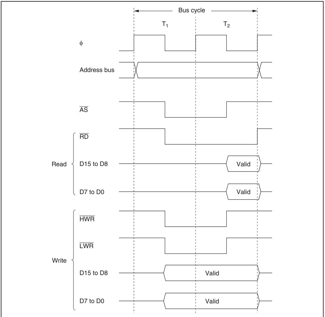
**Figure 7.9 Bus Timing for 16-Bit, 2-State Access Space
