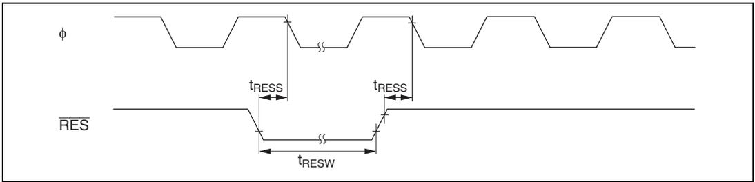
**Figure 23.4 Reset Input Timing**
