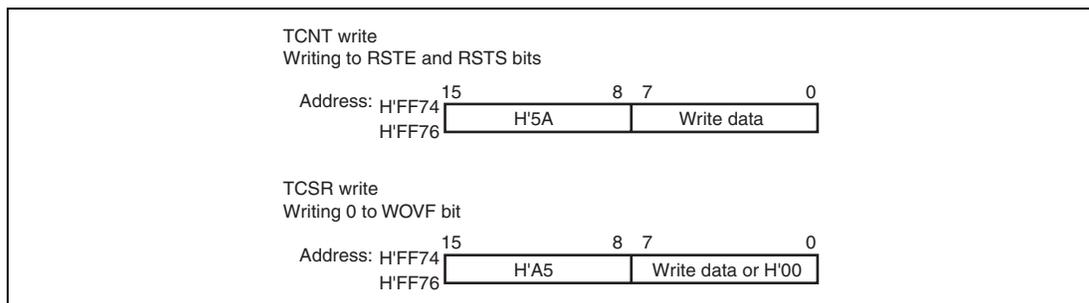
**Figure 12.4 Writing to TCNT, TCSR, and RSTCSR (example for WDT0)**
