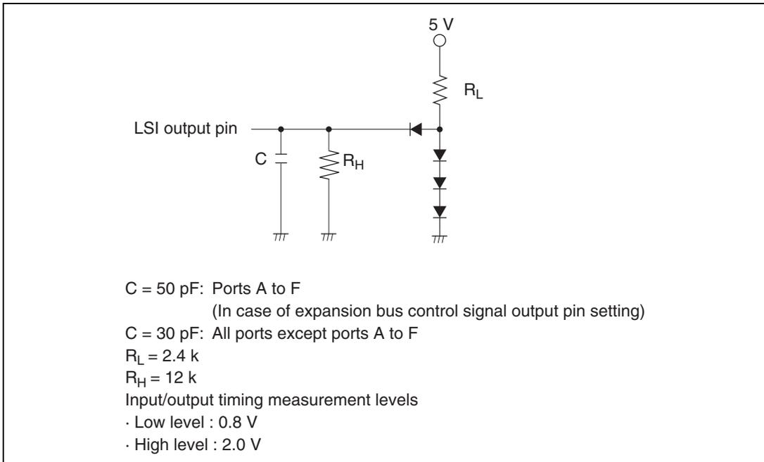
**Figure 23.1 Output Load Circuit**
