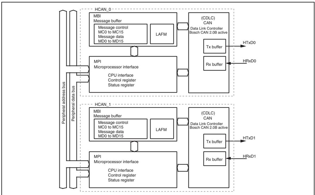
**Figure 14.1 HCAN Block Diagram**
