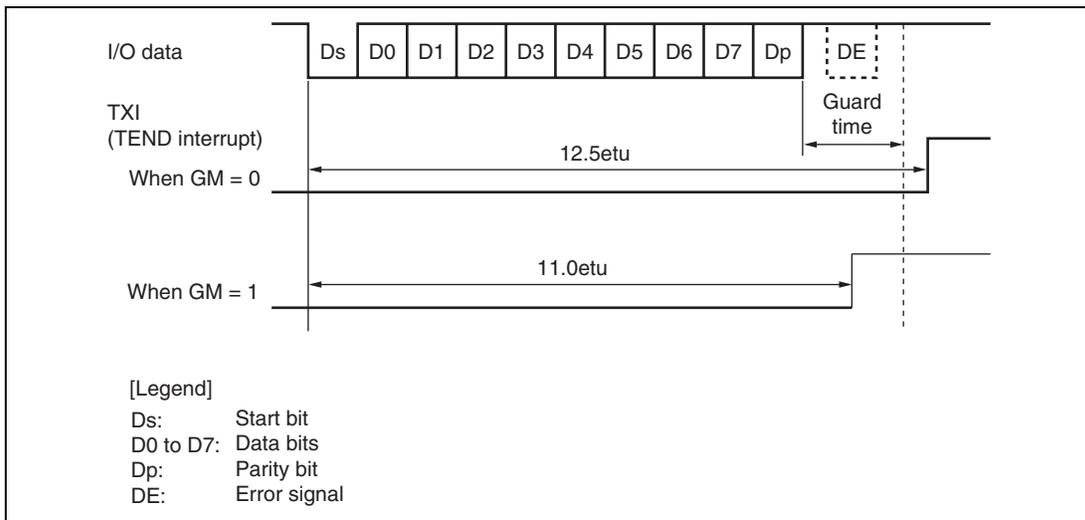
**Figure 13.27 TEND Flag Generation Timing in Transmission Operation**
