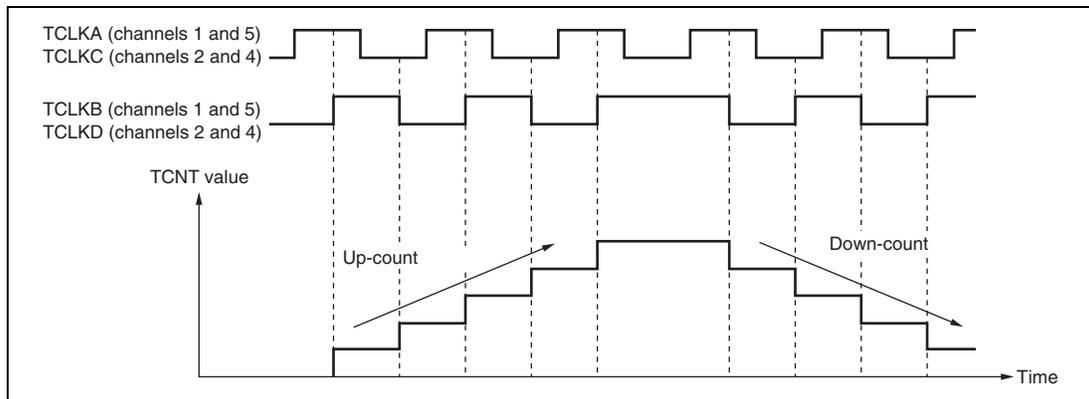
**Figure 10.28 Example of Phase Counting Mode 4 Operation**
