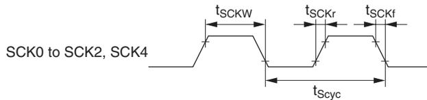
**Figure 23.16 SCK Clock Input Timing**
