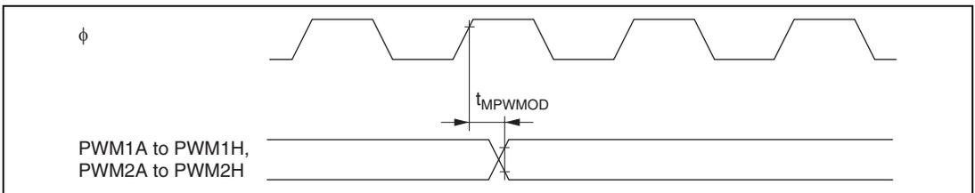
Figure 23.15 Motor Control PWM Output Timing
