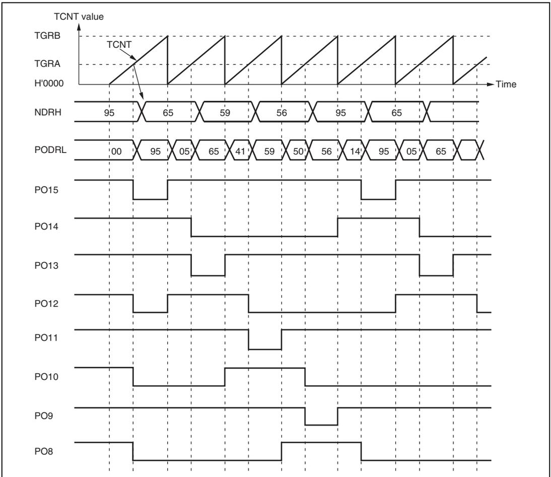
**Figure 11.10 Inverted Pulse Output (Example)**
