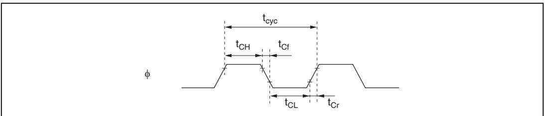
**Figure 23.2 System Clock Timing**
