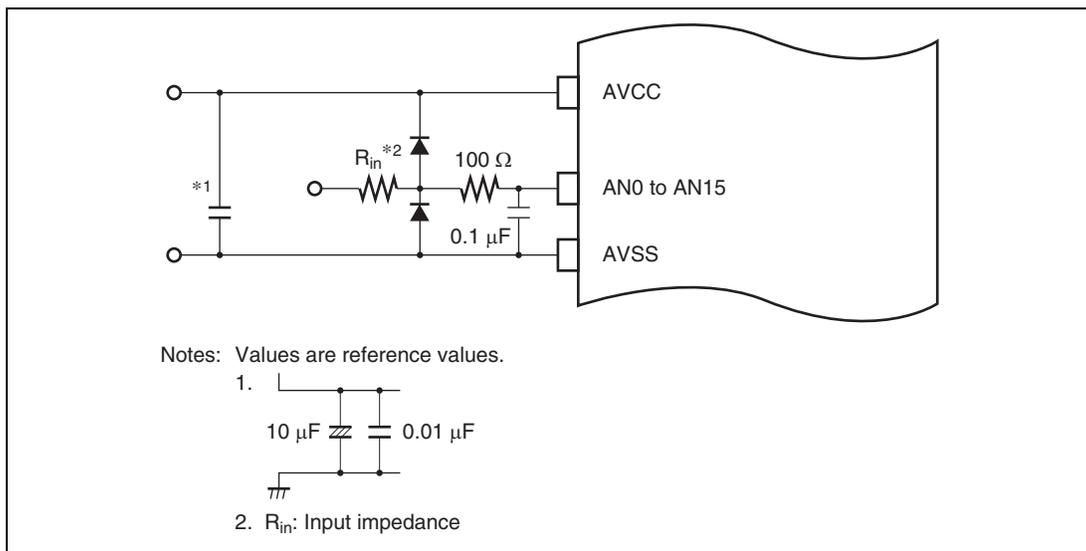
**Figure 15.7 Example of Analog Input Protection Circuit**
