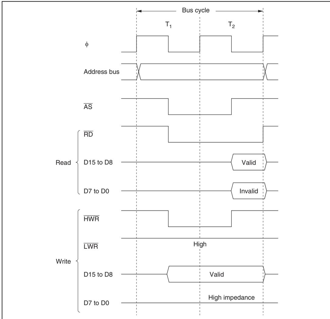
**Figure 7.5 Bus Timing for 8-Bit, 2-State Access Space**
