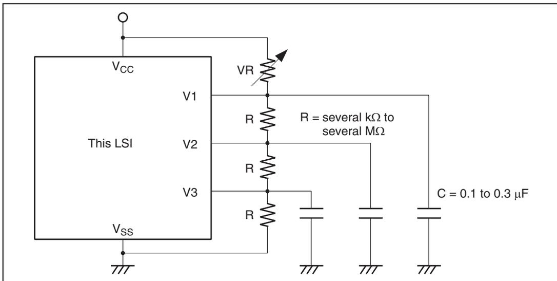
**Figure 17.9 Connection of External Split-Resistance**
