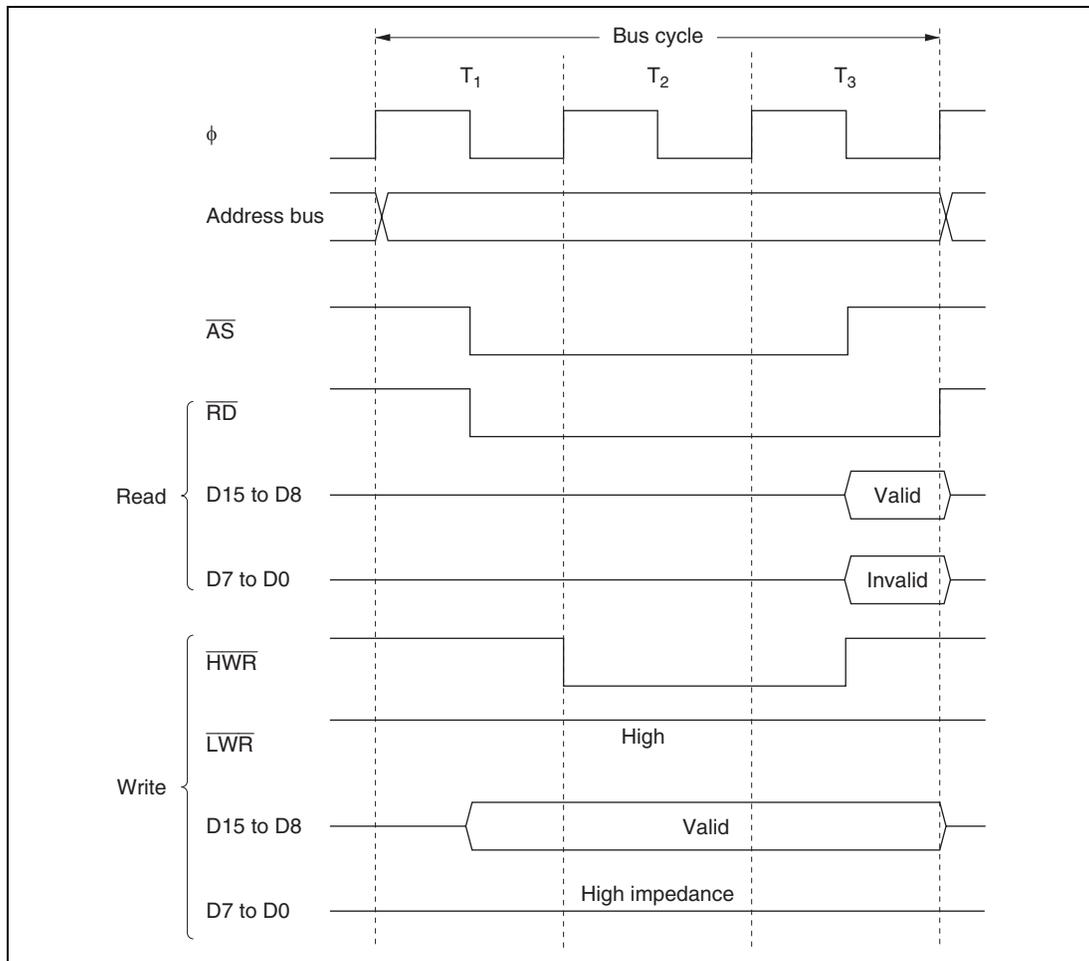
**Figure 7.10 Bus Timing for 16-Bit, 3-State Access Space
