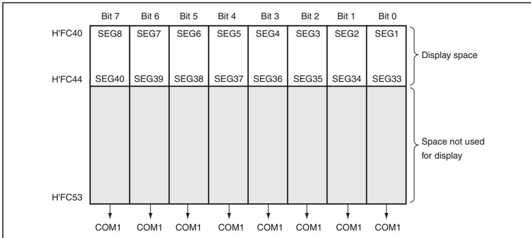
**Figure 17.6 LCD RAM Map (Static Mode)**
