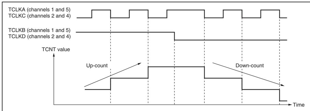
**Figure 10.26 Example of Phase Counting Mode 2 Operation**
