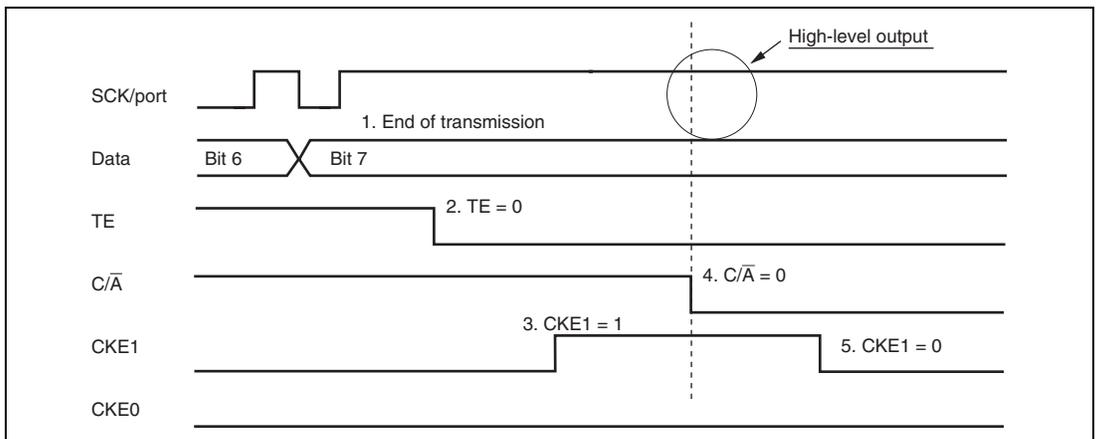
**Figure 13.39 Operation when Switching from SCK Pin to Port Pin
