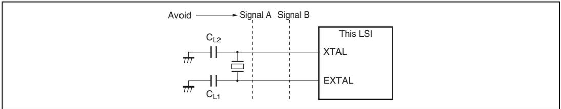
**Figure 20.9 Note on Board Design of Oscillator Circuit**
