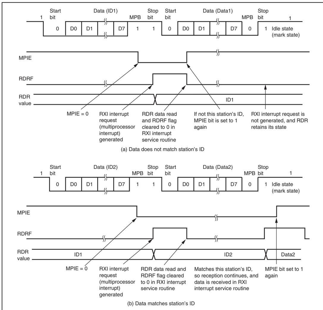
**Figure 13.12 Example of SCI Operation in Reception
