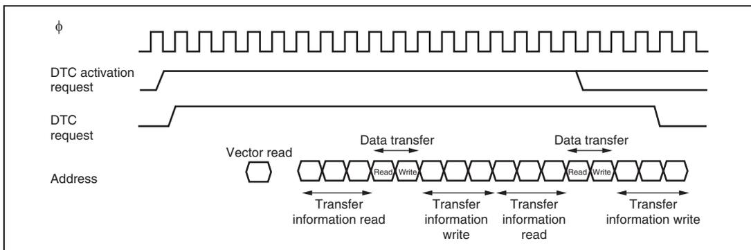
**Figure 8.11 DTC Operation Timing (Example of Chain Transfer)**
