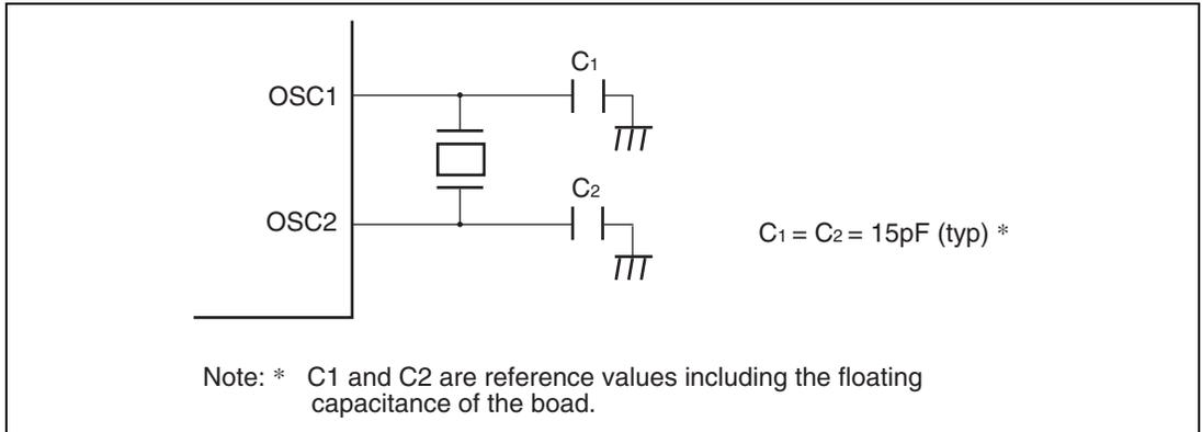
**Figure 20.6 Connection Example of 32.768-kHz Crystal Resonator**
