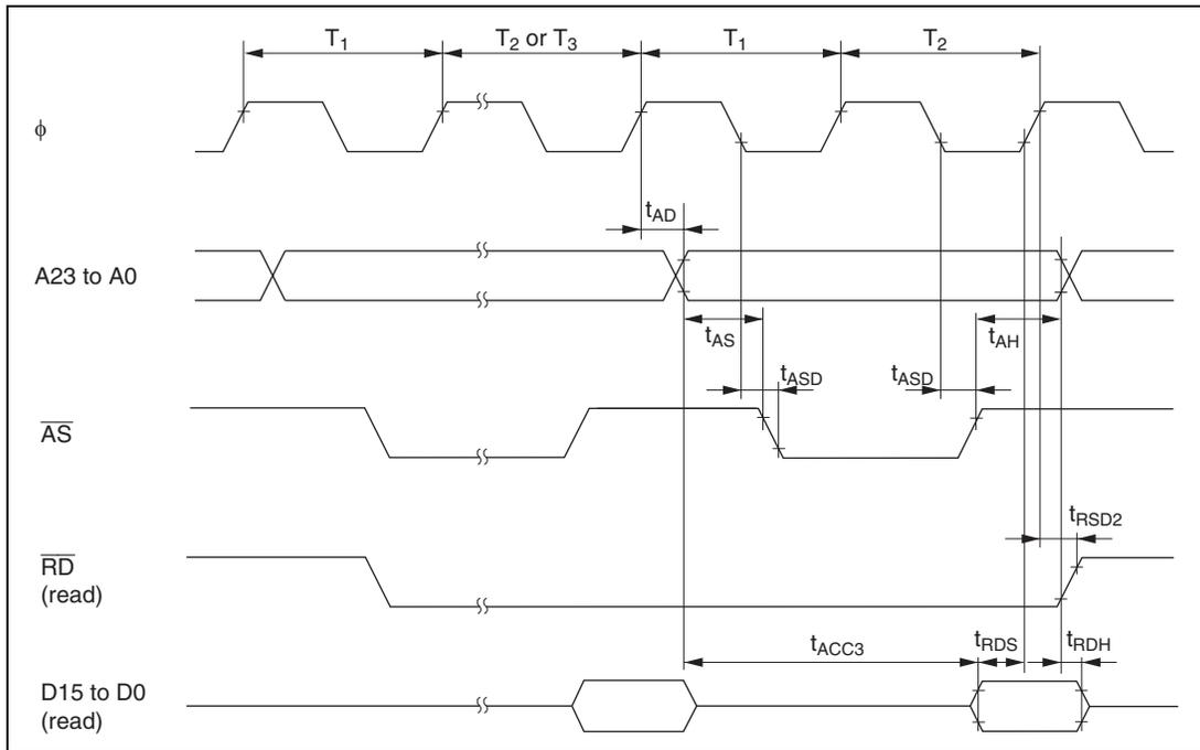
**Figure 23.9 Burst ROM Access Timing (Two-State Access)**
