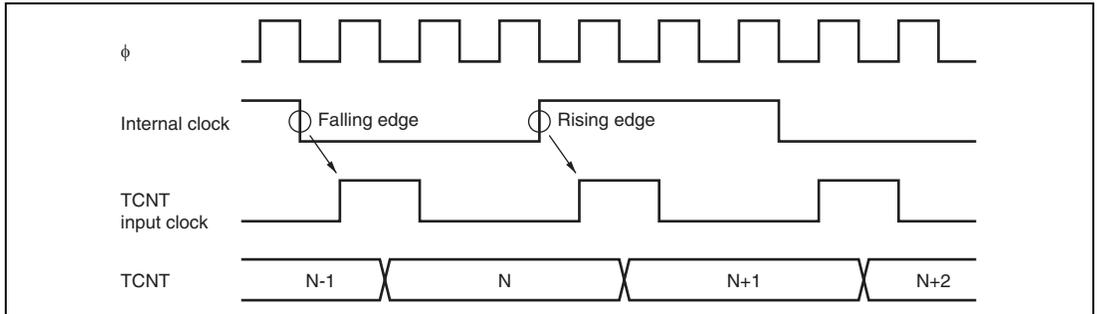
**Figure 10.30 Count Timing in Internal Clock Operation**
