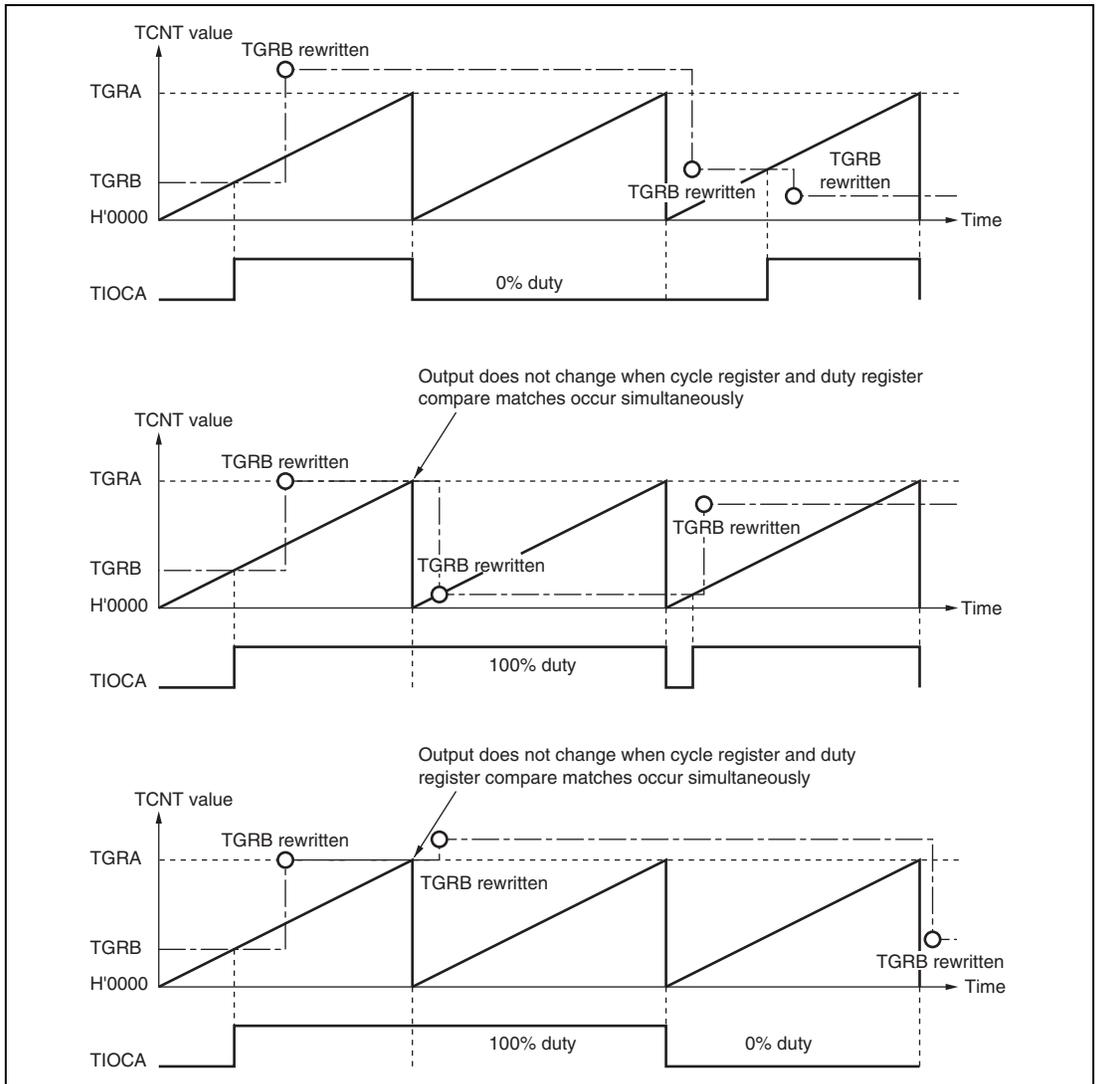
**Figure 10.23 Example of PWM Mode Operation (3)**
