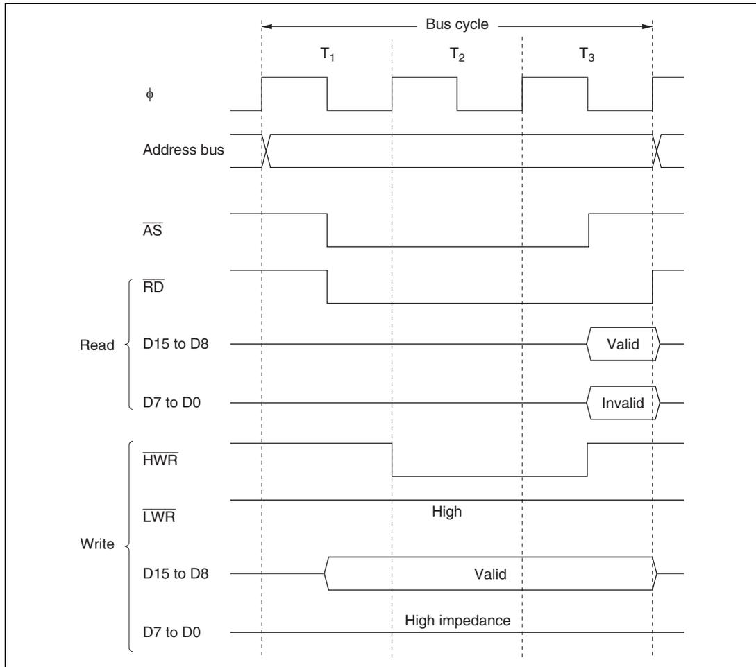
**Figure 7.6 Bus Timing for 8-Bit, 3-State Access Space**
