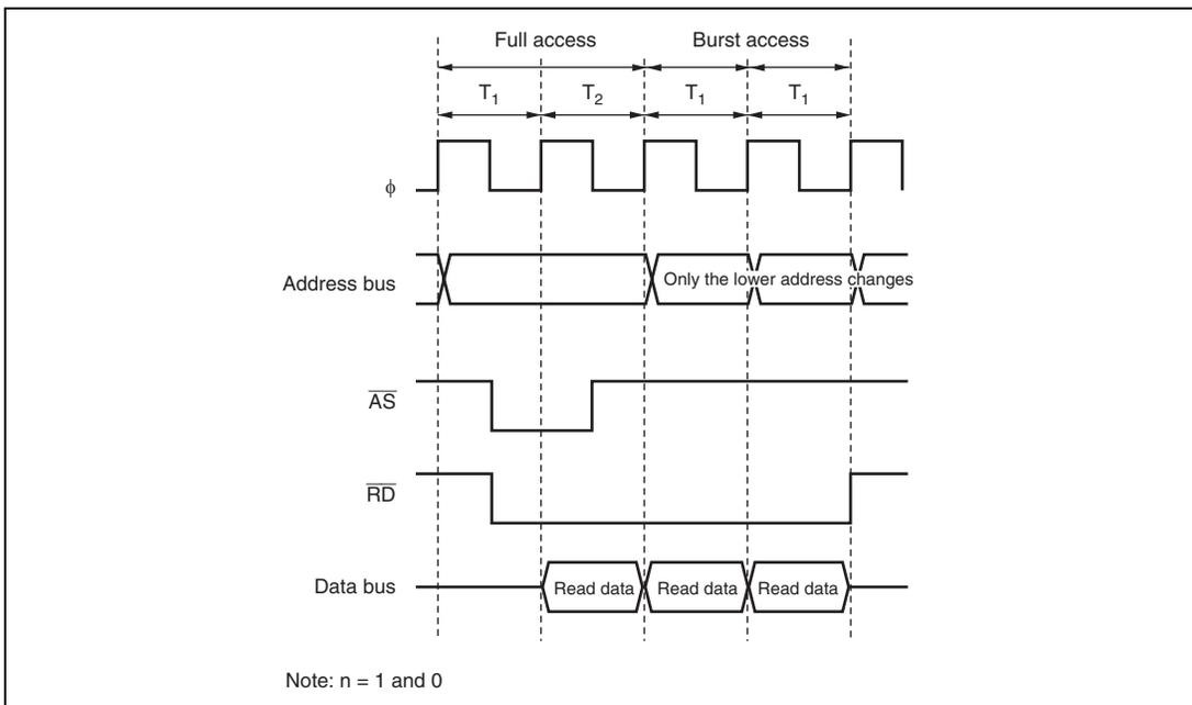
**Figure 7.15 Example of Burst ROM Access Timing**
