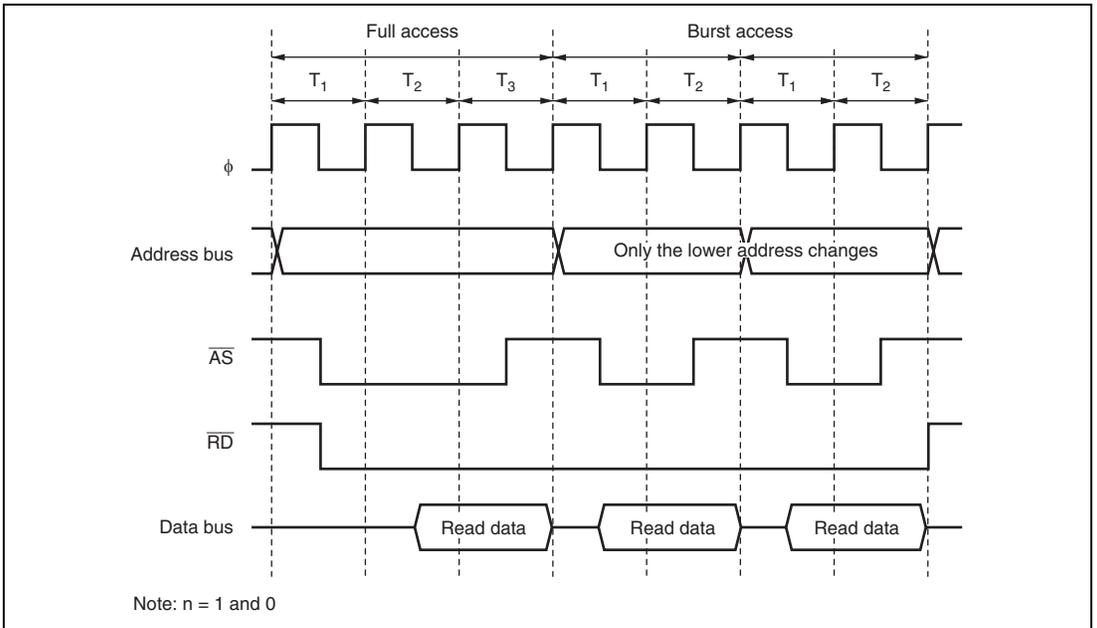
**Figure 7.14 Example of Burst ROM Access Timing**
