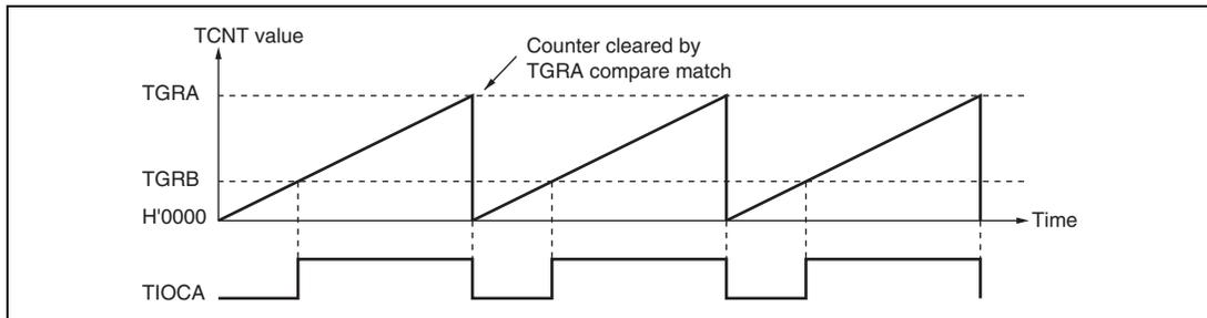
**Figure 10.21 Example of PWM Mode Operation (1)**
