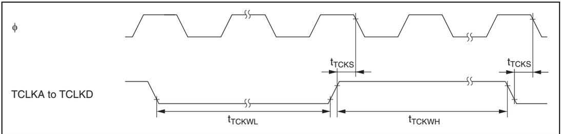
Figure 23.14 TPU Clock Input Timing
