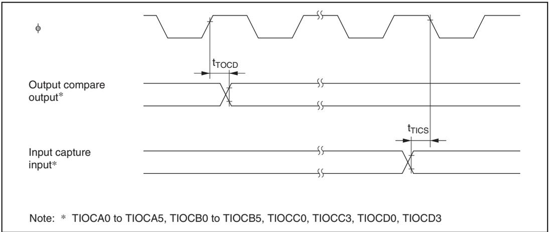
Figure 23.13 TPU Input/Output Timing
