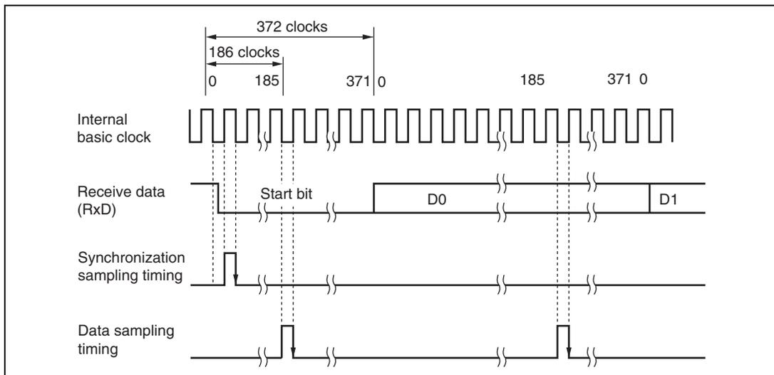
**Figure 13.25 Receive Data Sampling Timing in Smart Card Mode
