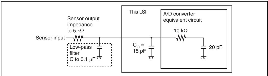
**Figure 15.6 Example of Analog Input Circuit**
