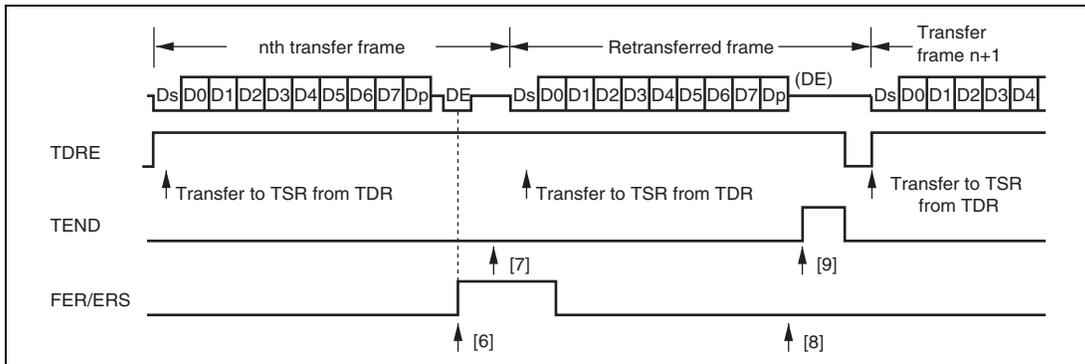
**Figure 13.26 Retransfer Operation in SCI Transmit Mode**
