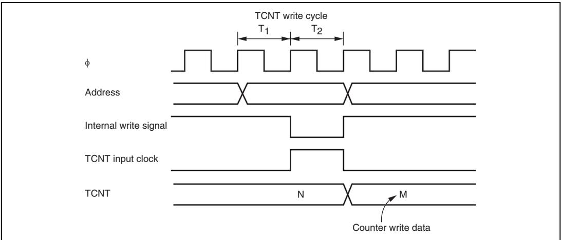
**Figure 12.5 Contention between TCNT Write and Increment**
