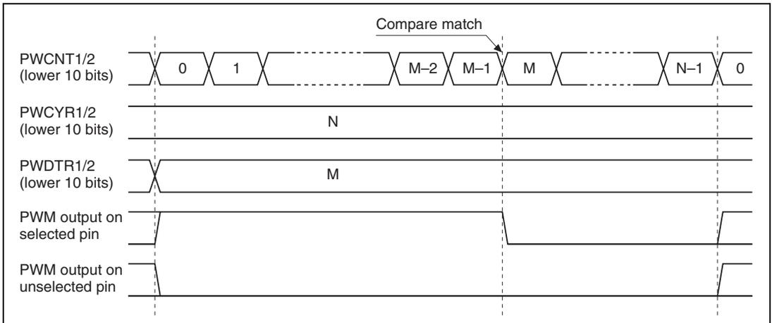
**Figure 16.3 Duty Register Compare Match (OPS = 0 in PWPR)**
