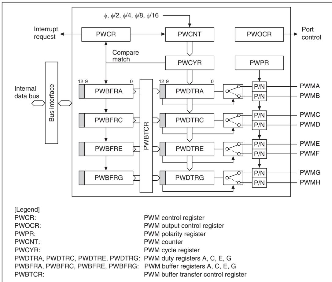
**Figure 16.1 Block Diagram of PWM**
