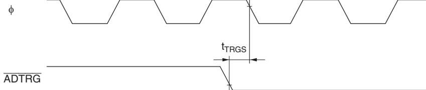
**Figure 23.18 A/D Converter External Trigger Input Timing**
