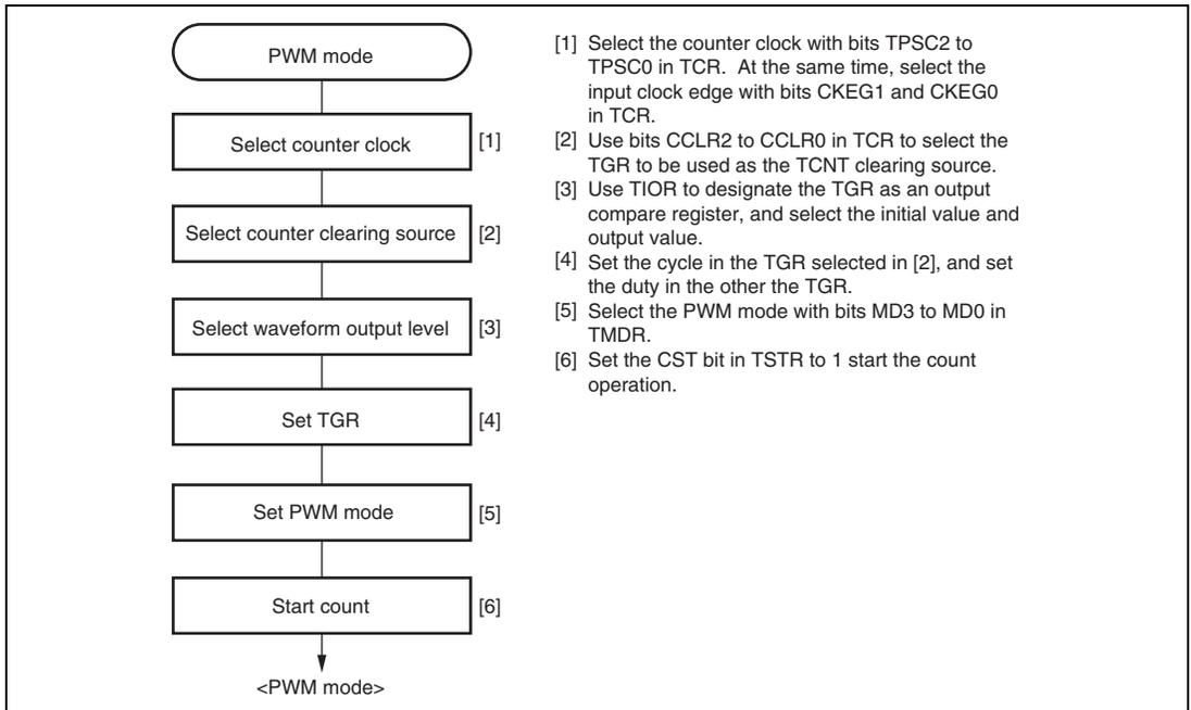
**Figure 10.20 Example of PWM Mode Setting Procedure**
