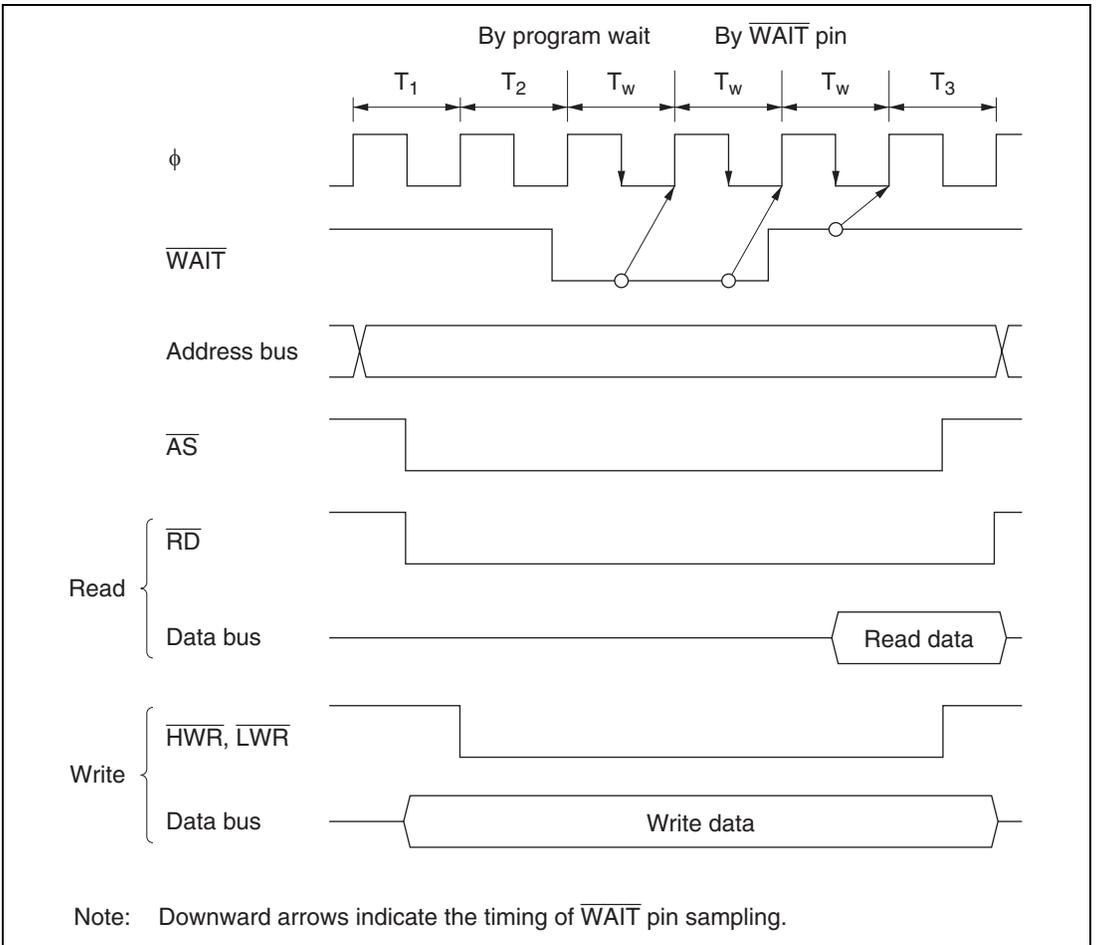
**Figure 7.13 Example of Wait State Insertion Timing**
