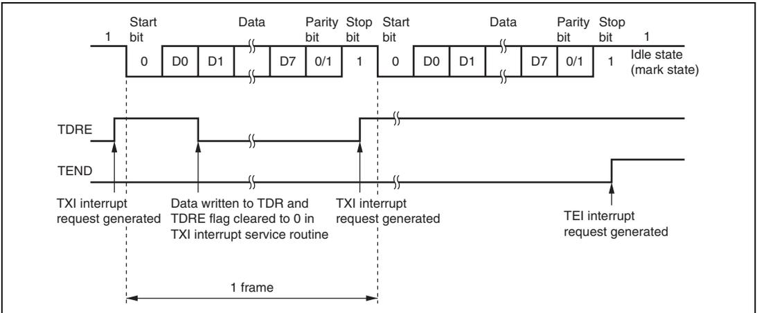
**Figure 13.6 Example of Operation in Transmission in Asynchronous Mode
