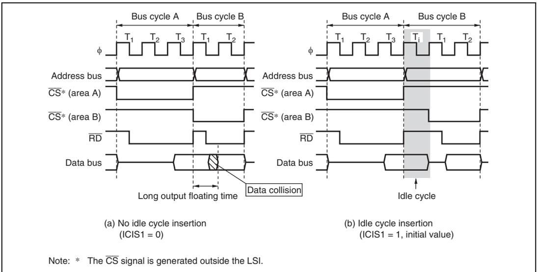
**Figure 7.16 Example of Idle Cycle Operation
