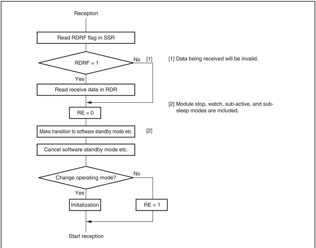
**Figure 13.37 Sample Flowchart for Mode Transition during Reception**
