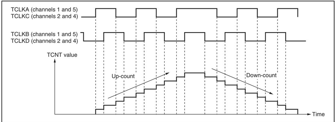
**Figure 10.25 Example of Phase Counting Mode 1 Operation**
