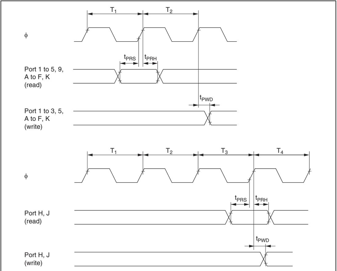
**Figure 23.11 I/O Port Input/Output Timing**
