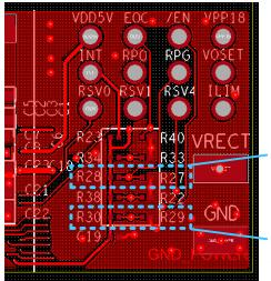
R28 and R27 on the RPPG Pin for RPP Gain Adjustment
