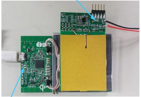
Solder wire leads to GND and VOUT test points to allow measuring VOUT or to apply load
