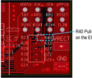
R40 Pull-Down Resistor on the EOC Pin
