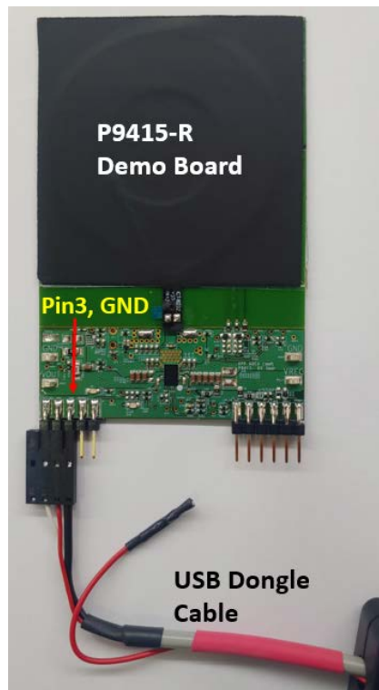
Figure 9. USB-I2C Bridge Connected to I2C Terminal J1 of P9415-R EVK Demo Board; USB Cable
