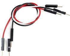
Figure 25. Two Male-to-Male Jumper Wires (Optional)
