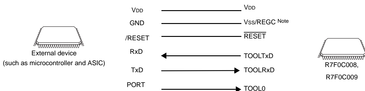
Figure 25 - 4 Communication with External Device
