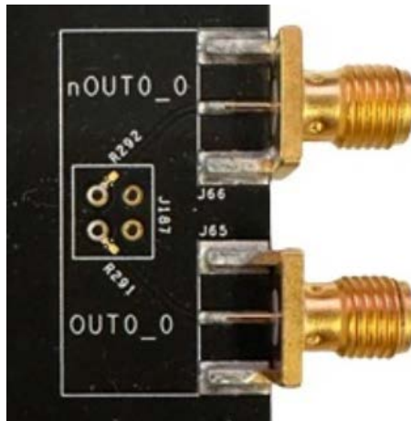
Figure 7. Differential Output Pair Example
