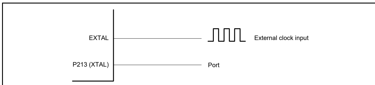
Figure 9.8 Equivalent circuit for external clock
