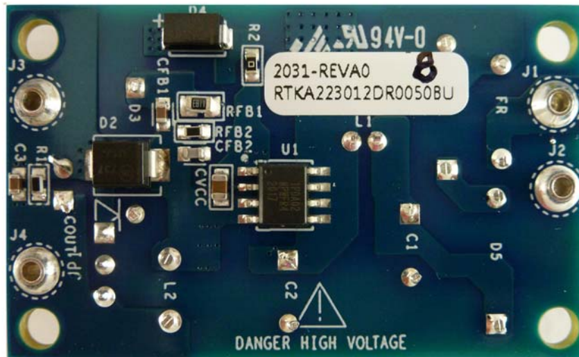
Figure 3. RTKA223012DR0050BU Evaluation Board (Bottom)
