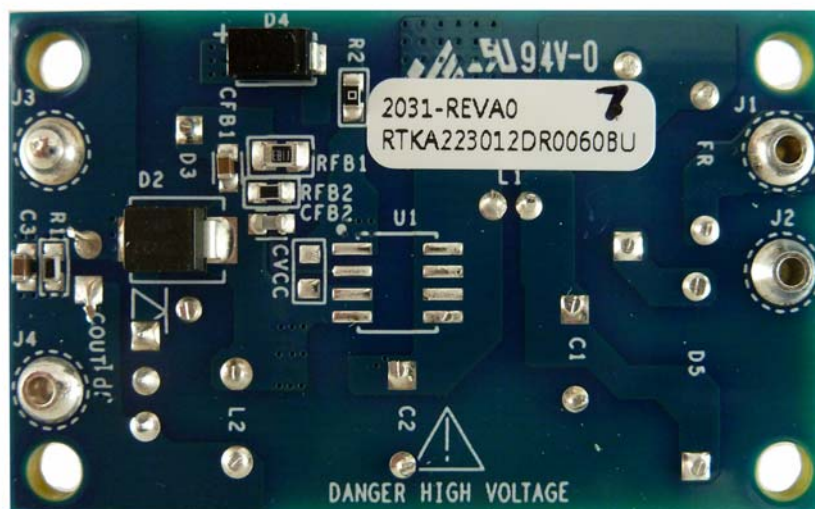
Figure 5. RTKA223012DR0060BU Evaluation Board (Bottom)
