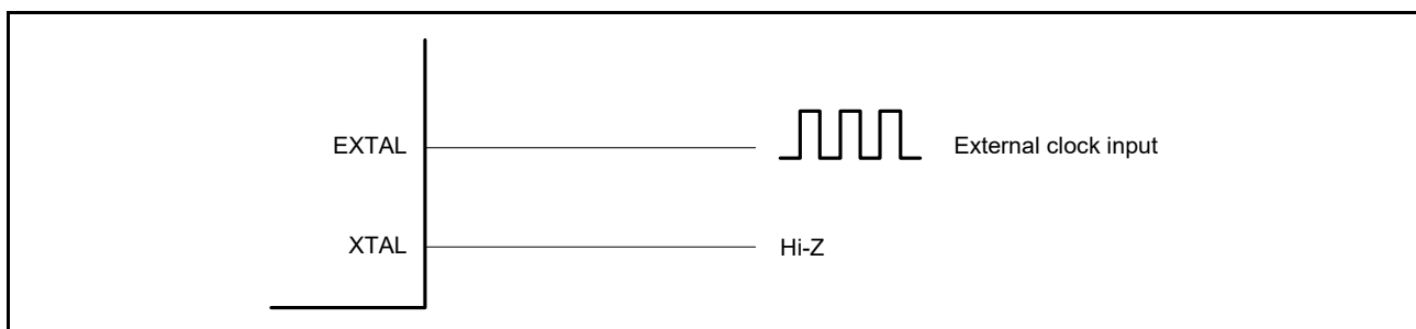
Figure 9.5 Equivalent circuit for external clock
