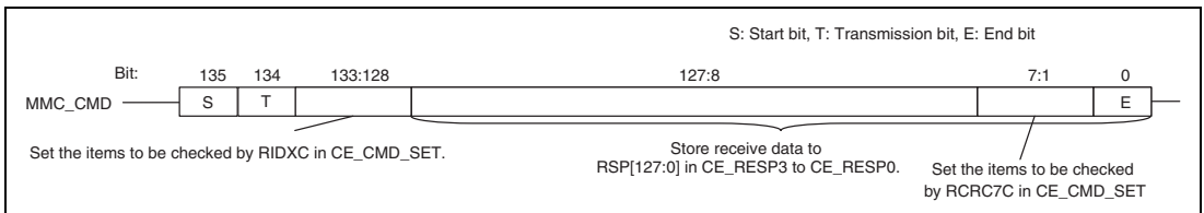
Figure 45.4 Format of 17-Byte Response (R2)
