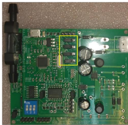
Figure 3-1 Program Development/Debugging Using JLINK on RA2L1 CAN Sensor EVB
