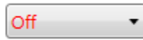
Figure 20. Example of a Modified Value that is Not Yet Saved to Memory
