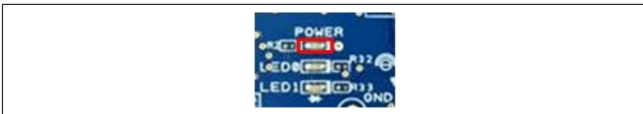
Figure 11. Power LED on EK-RA4W1 Board
