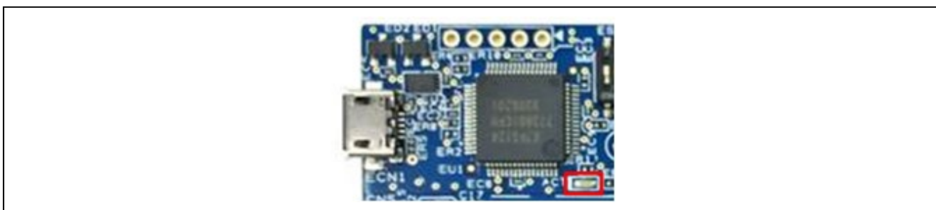
Figure 10. ACT LED on EK-RA4W1 Board
