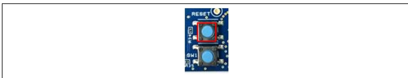
Figure 16. Reset Switch on EK-RA4W1 Board
