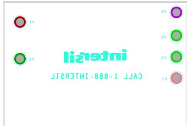
FIGURE 4. ISL6844EVAL3Z - BOTTOM LAYER (SILKSCREEN)
