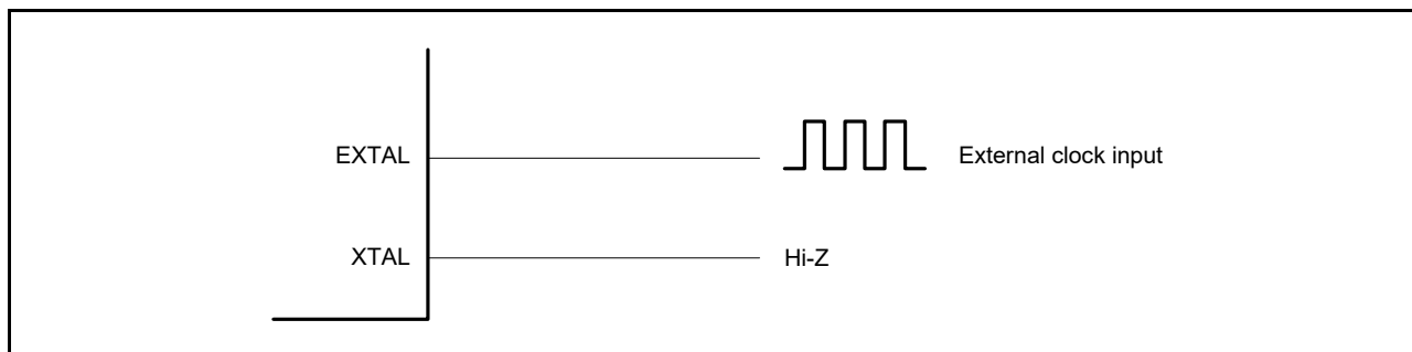
Figure 9.5 Equivalent circuit for external clock
