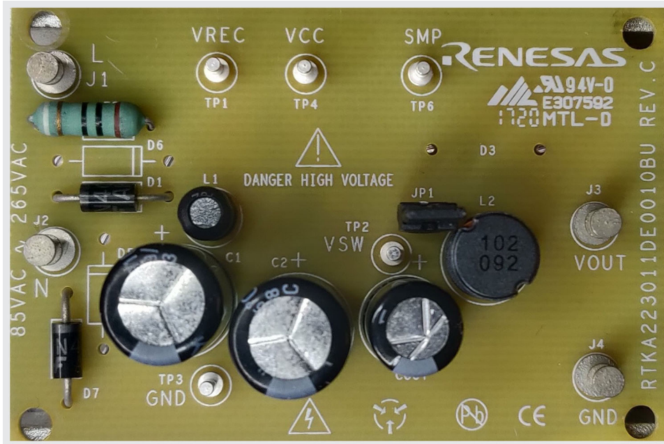
Figure 2. RTKA223011DE0010BU Evaluation Board (Top)
