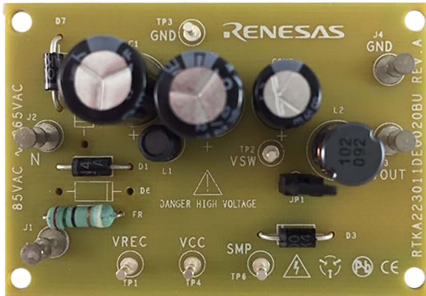
Figure 2. RTKA223011DE0020BU Evaluation Board (Top)
