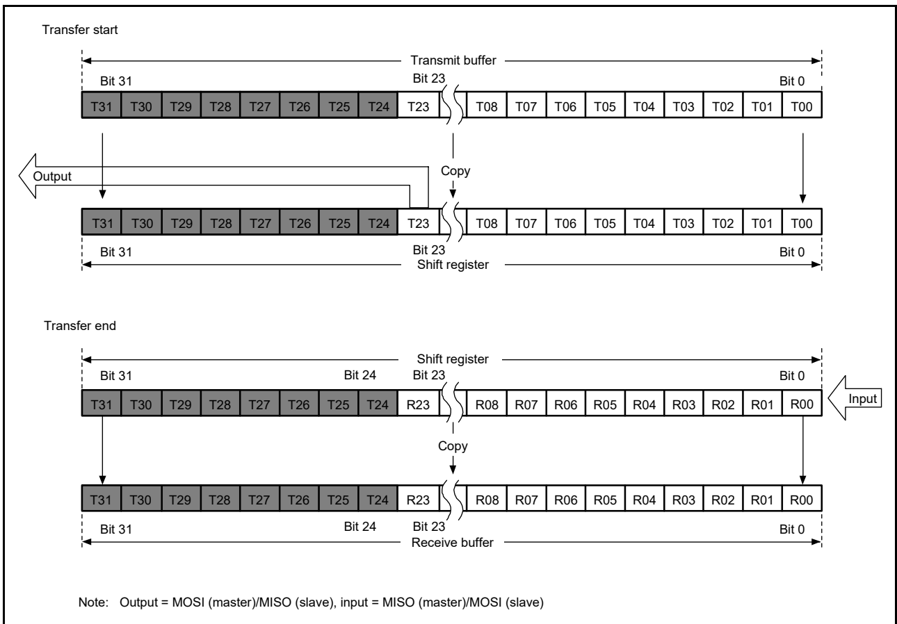
Figure 38.15 MSB First Transfer (24-Bit Data, Parity Disabled)
