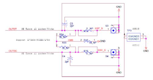
The circuit is designed for maximum flexibility when testing all possible logic types. Default assembly uses a 0.1µF capacitor in place of R14 and R16, and the short across R14 and R16 is cut. No other devices are assembled. This simple AC-coupled configuration allows for testing phase noise and jitter of all possible logic types. The circuit can be modified for custom tests. TP3 is a position to place a differential FET probe.
