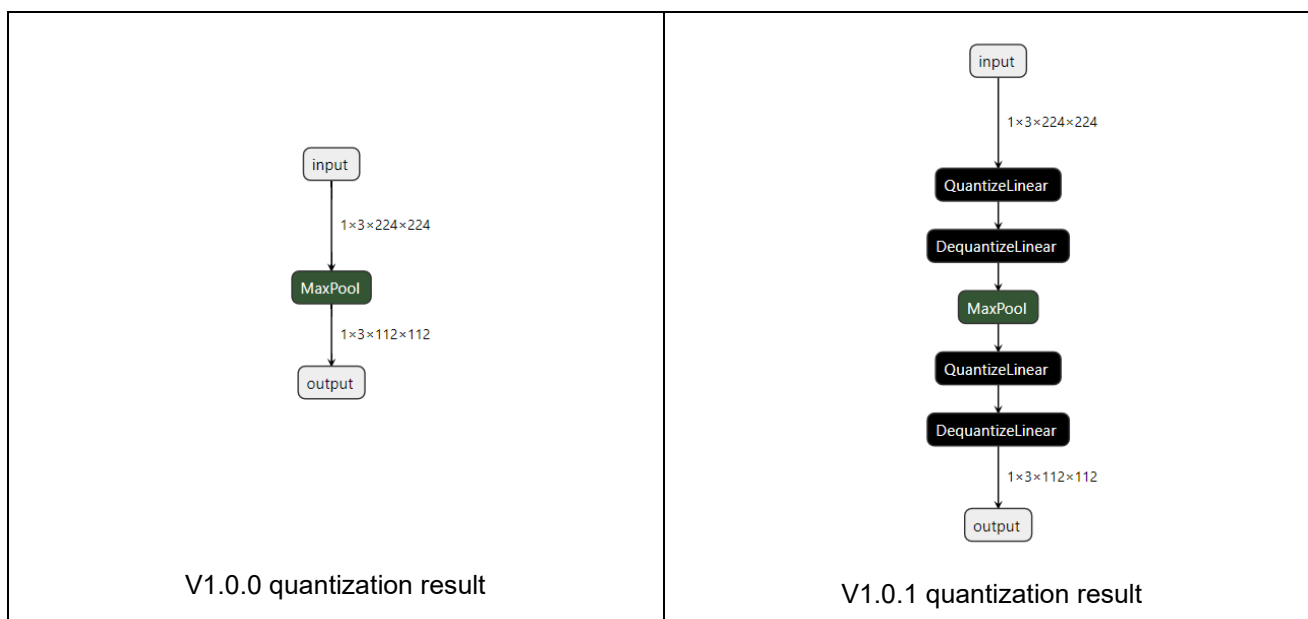
Figure 1.3 In Version v1.01, When the `maxpool` node is the initial or final layer, It will also be quantized
