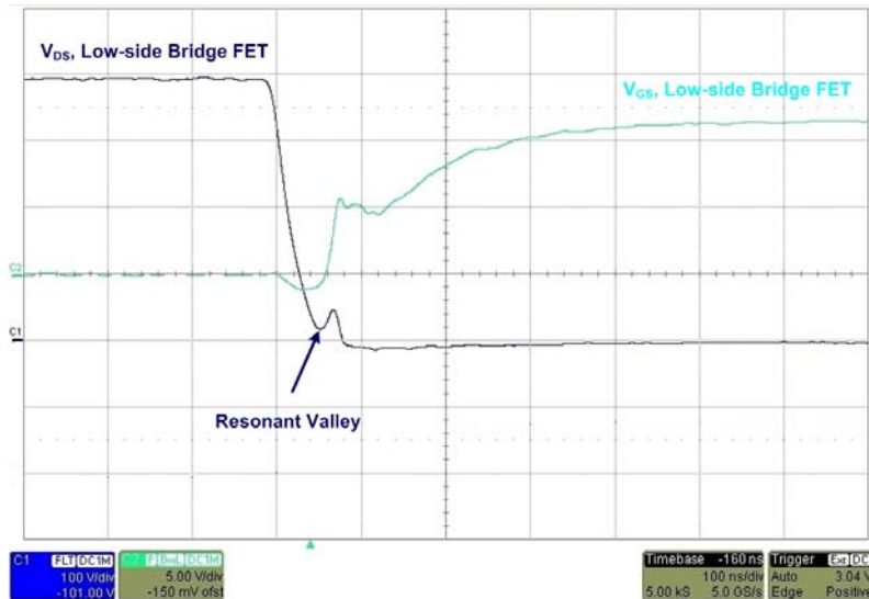
FIGURE 21. RESONANT SWITCHING WITH 100% (50A) LOAD
