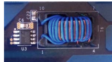
FIGURE 9. PULSE TRANSFORMER AND DRIVER
