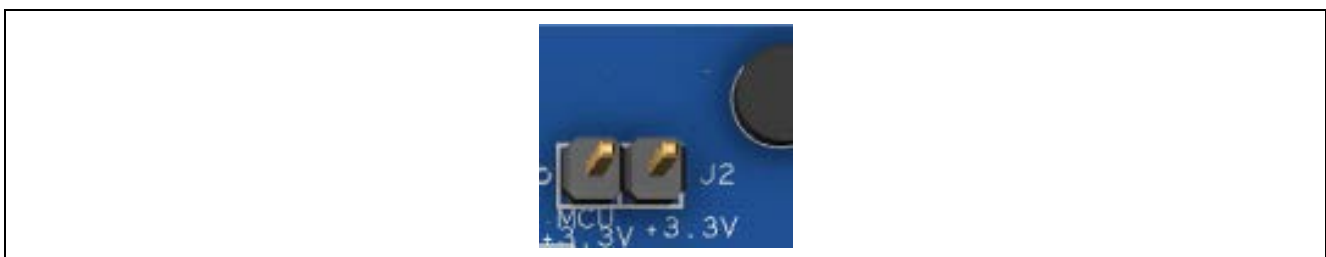
Figure 20. RX MCU Current Measurement
