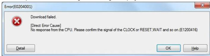
In order to avoid this error, open the RL78 E1 (Serial) Property, and set the "Erase flash ROM when starting" on the Connect Settings tab to YES, to download the program.
