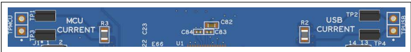
Figure 26. RA MCU Current Measurement
