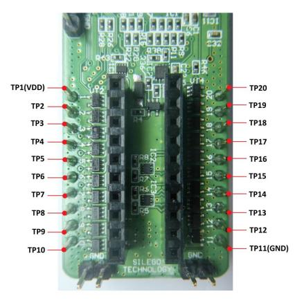
**Figure 4: Expansion Connector Pinout**
