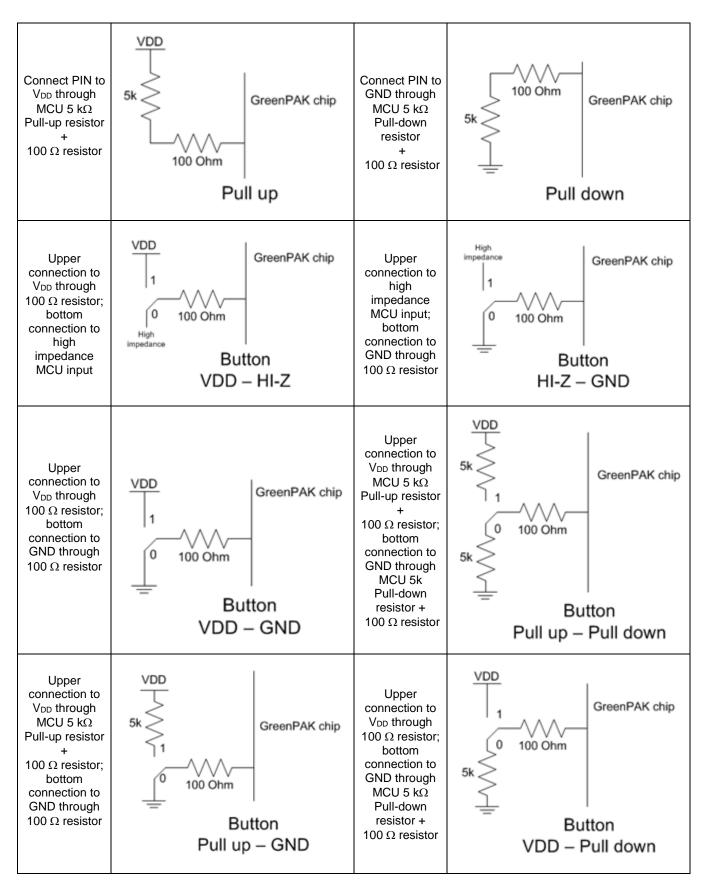
Figure 6 shows the schematic connection of the GP  $V_{DD}$  pins.
