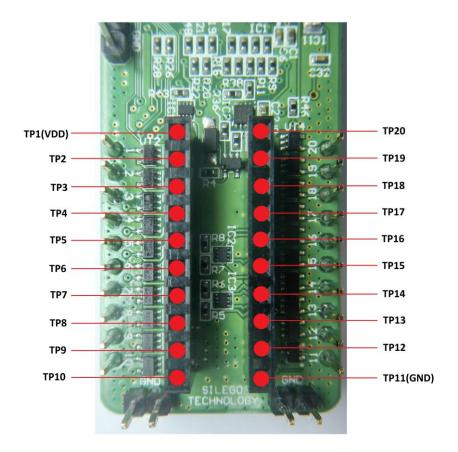
Figure 2: DIP Adapter Connector Pinout
