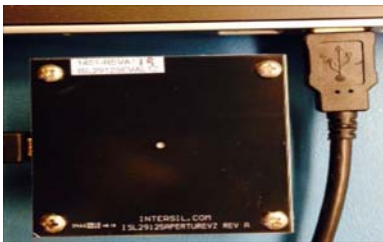
FIGURE 43. PC TO EVALUATION BOARD CONNECTION
