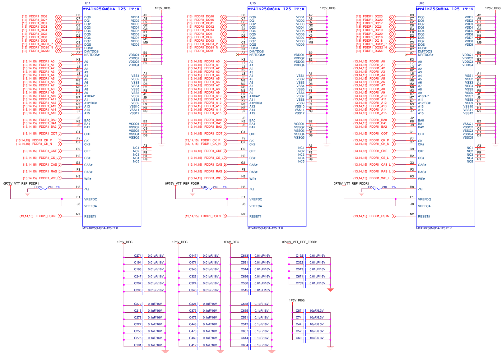
Figure 16. Schematic - DDR3-SDRAM Interface 1 - FDDR1
