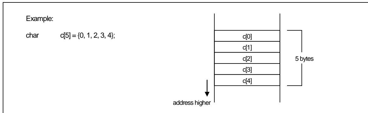
Figure D.3 Example of Placement of Array
