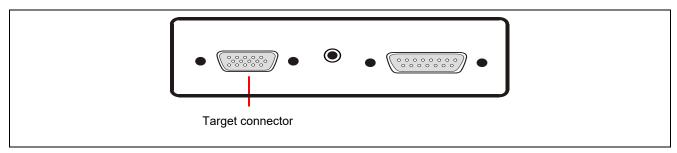
Figure 10.8 Target Connector (Target Connector Side of the FP6)
