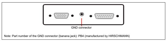
Figure 10.13 GND Connector (Target Connector Side of the FP6)
