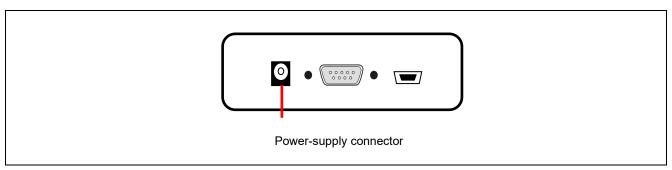
Figure 10.1 Power-Supply Connector
