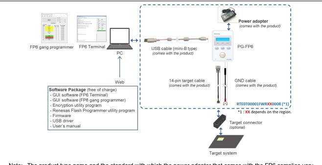
Note: The product type name and the standard with which the power adapter that comes with the FP6 complies vary with the region where it is to be used. Be sure to use the power adapter that is appropriate for your region.
