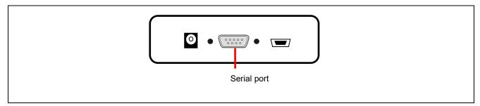
Figure 10.3 9-Pin D-Sub Serial Connector
