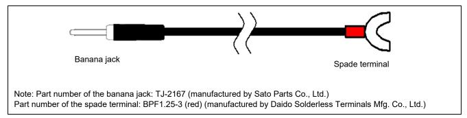
Figure 10.14 Appearance of the GND Cable
