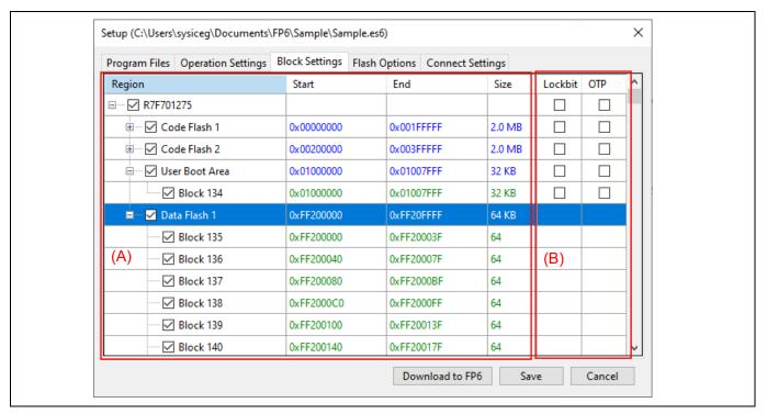
Figure 4.8 [Block Settings] Tabbed Page (Case of Other Device Types)
