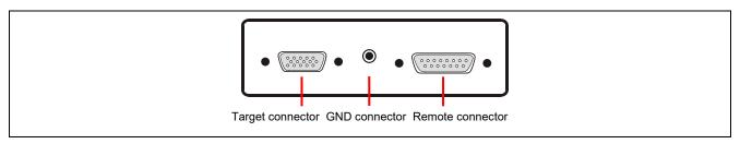
Figure 2.4 FP6 Target Connector Side
