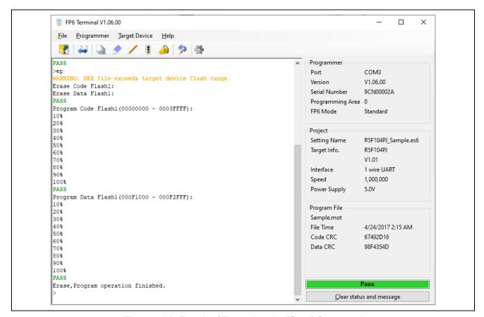
Figure 4.32 Result of Executing the [Start] Command
