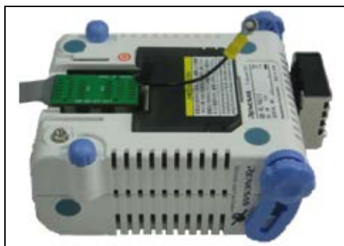
Figure 2-7. Connect the QB-RL78G1F to the probe
