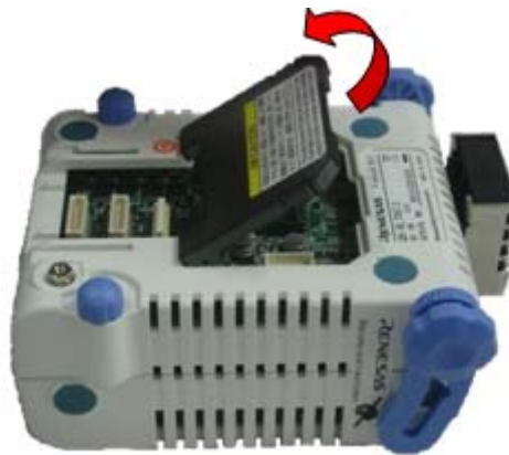
Figure 2-1. Acrylic Board Removal Method
