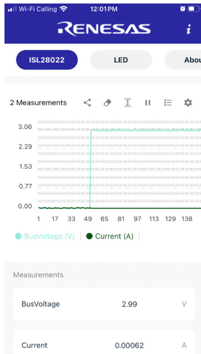
Figure 31. Bus Voltage and Current Reading
