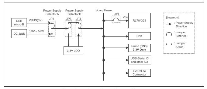
Figure 2-5. **Power Source System Diagram**
