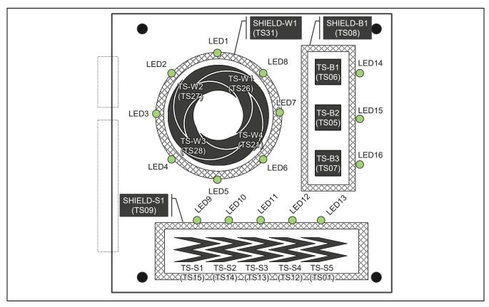
Figure 2. Board Layout and TS Pin Assignments
