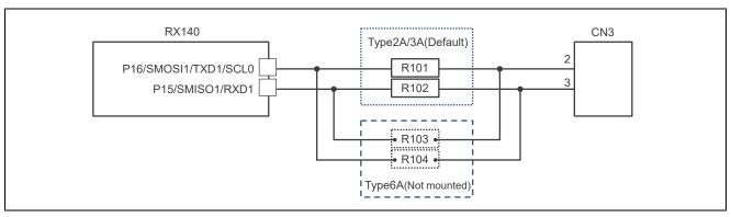
Figure 1-1. Pmod™ Interface Switch Circuit
