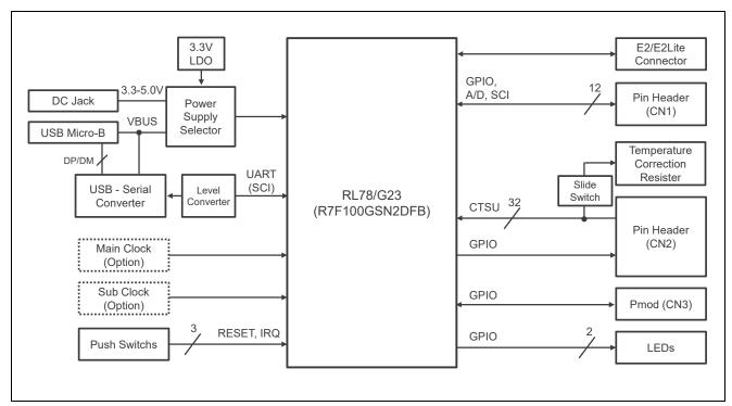
Figure 2-1. System Block Diagram
