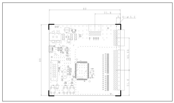
Figure 2-3. RL78/G23 Cap Touch CPU System Board Dimensions
