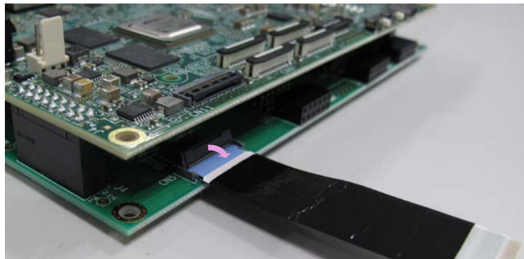
Figure 2.1-1 Connect FFC to RZ/V2H EVK Expansion Board
