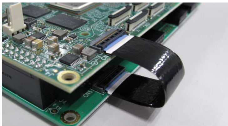
Figure 2.1-2 Connect FFC to RZ/V2H Secure Evaluation Board
