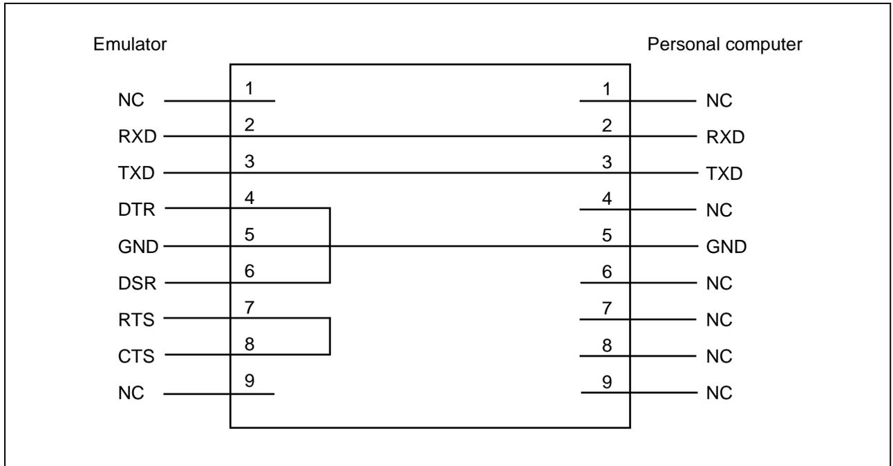
**Figure 6.2 Testing Circuit for SERIAL I/F Test**
