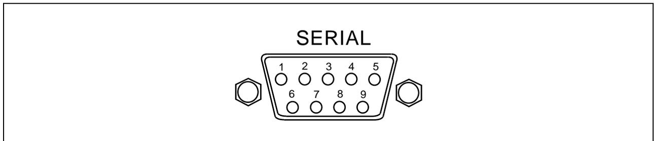
**Figure 6.3 Pin Locations in E8000 Emulator Serial Interface Connector**
