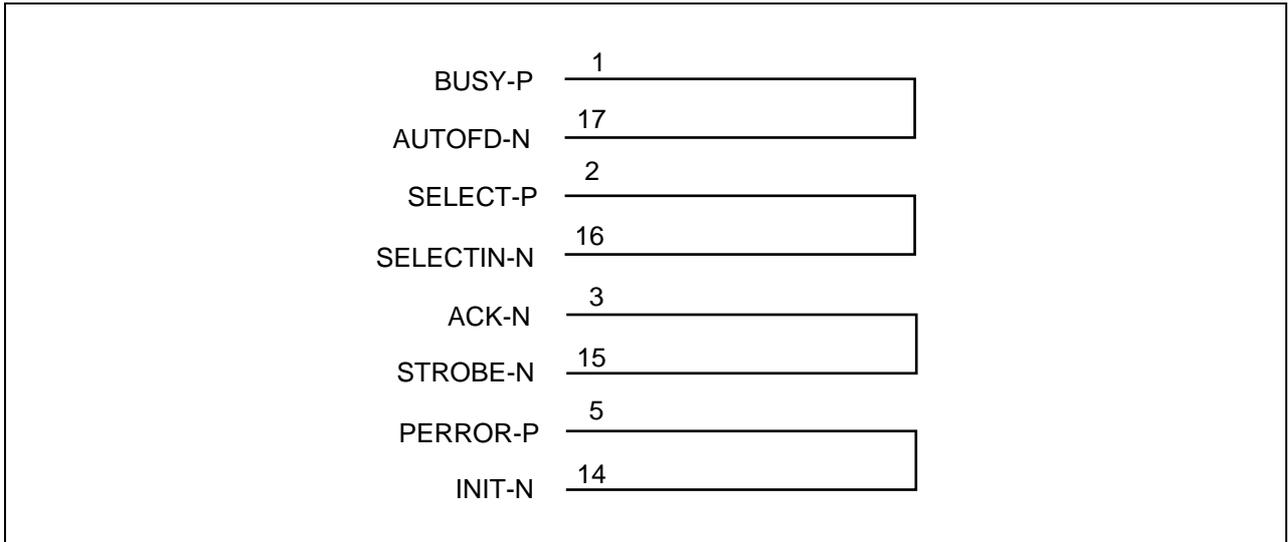
**Figure 6.1 Testing Circuit for P1284 Loop Back Test**
