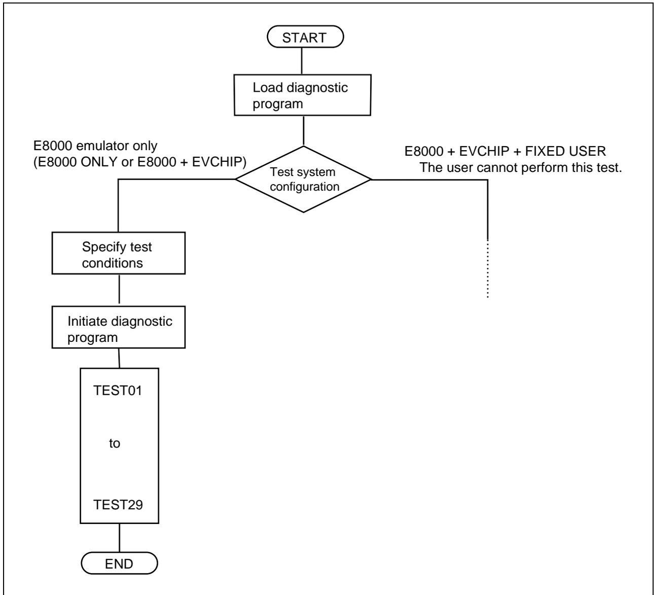
**Figure 3.1 Diagnostic Program Operation Flowchart**
