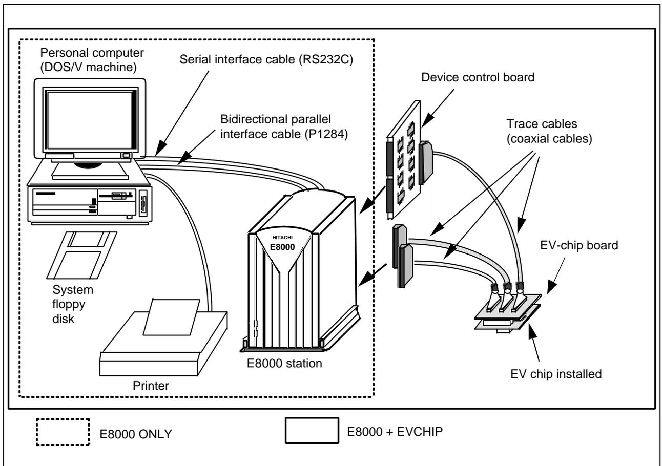
**Figure 2.1 Test System Configuration**
