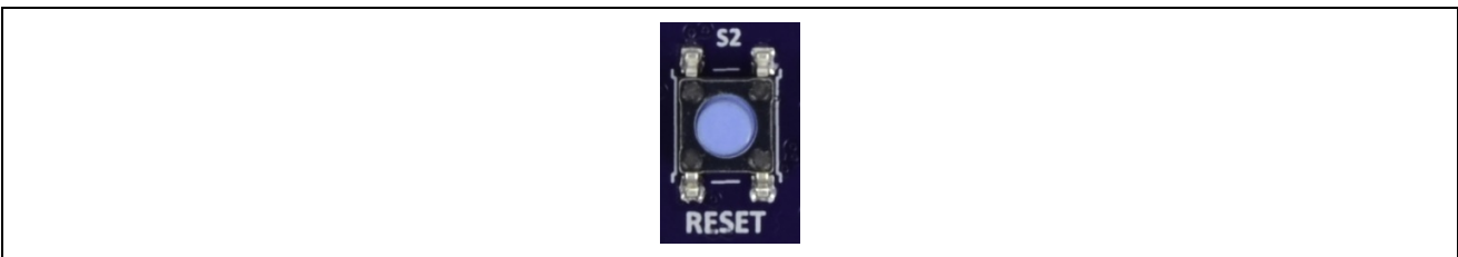
Figure 18. Reset Switch (S2) on Target Board
