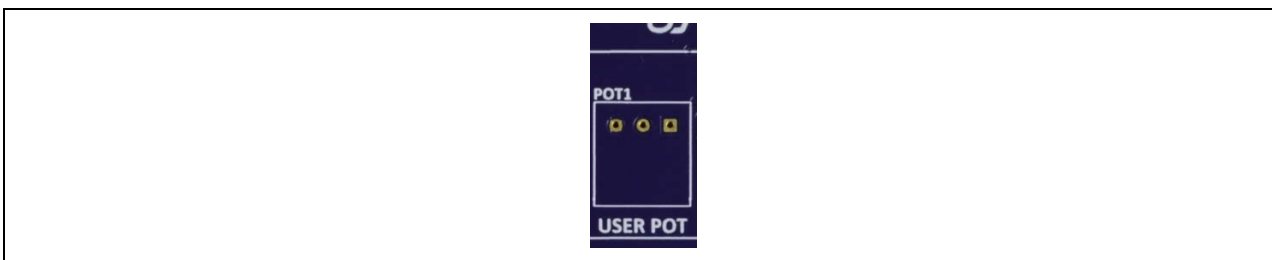
Figure 30. User Potentiometer on Target Board (Top)
