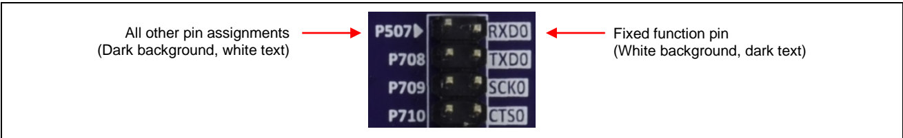
Figure 22. Fixed Function Pin Label Example
